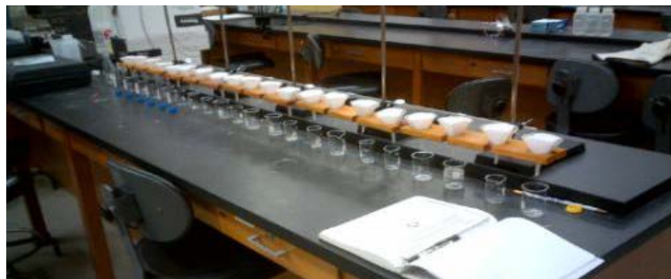
Figure 8 Staging samples to measure Conductivity and pH
