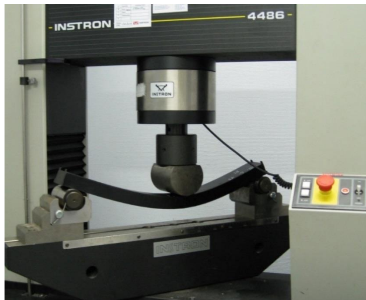
Figure 8: Flexural test with 3-point loading [21]
