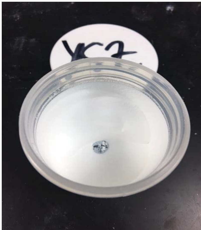
Figure 3.2. Printable YSZ paste (particles are well suspended without any presence of segregation or agglomeration)
