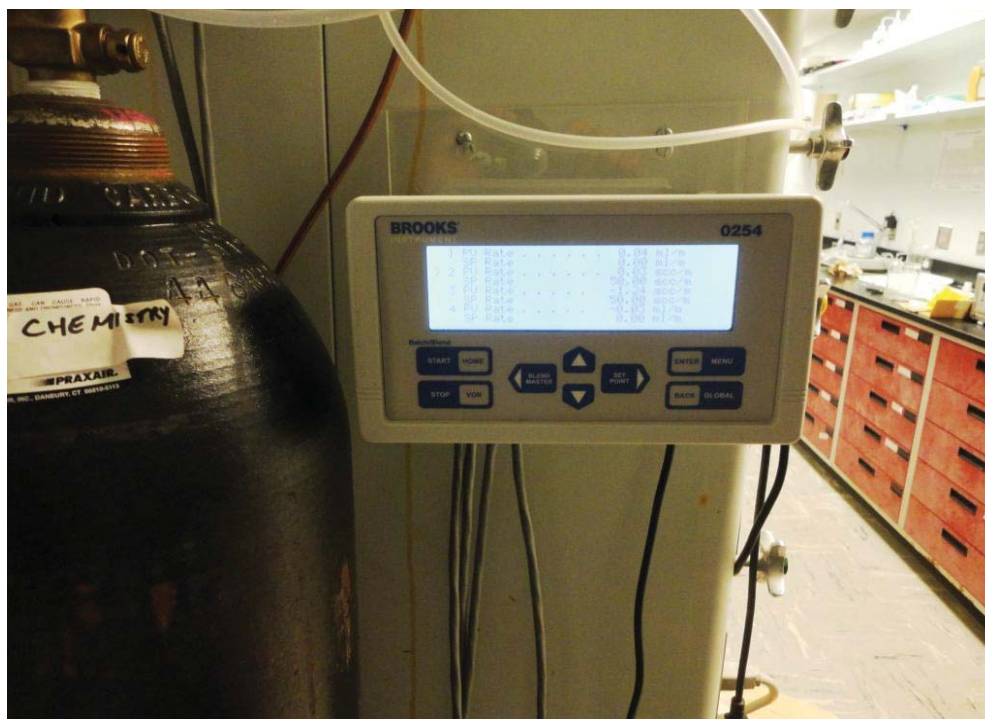
Figure A.11. Mass flow controller module; can control up to 4 gas flows simultaneously
