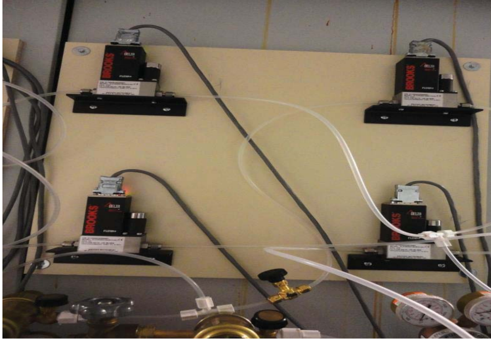
Figure A.12. Flow meters can control up to 100 mL/min
