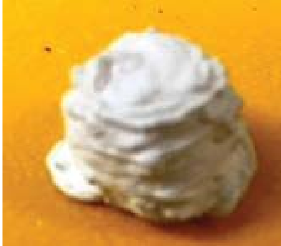
Figure 4.11. 3d-printed YSZ cube using water as the solvent and 3% methoxy cellulose as the binder.
