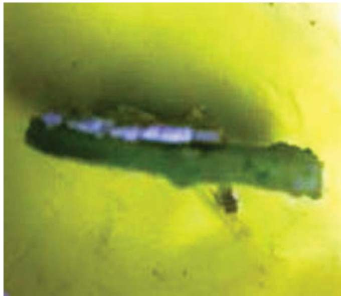
Figure 4.29. Side view of delamination caused by mismatch of shrinkage of YSZ and Ni-YSZ.
