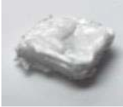
Figure 4.17. YSZ square wafer printed with paste containing 3% methyl cellulose as the binder and water as the solvent
