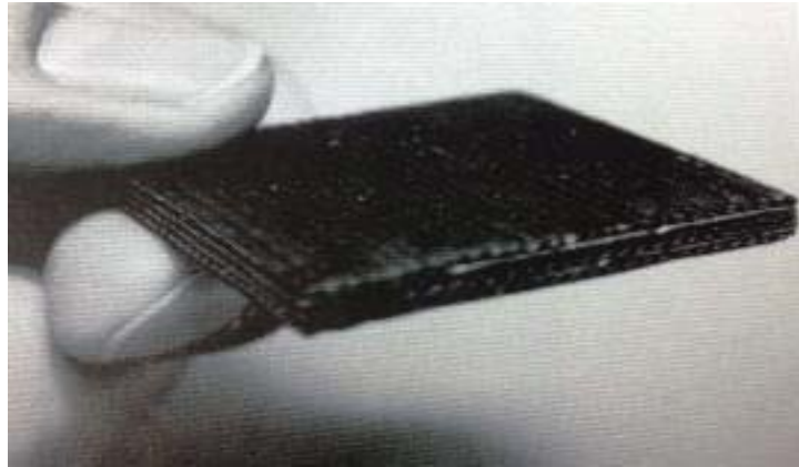
Figure 1.15 Monolithic cell fabricated by tape casting [33]
