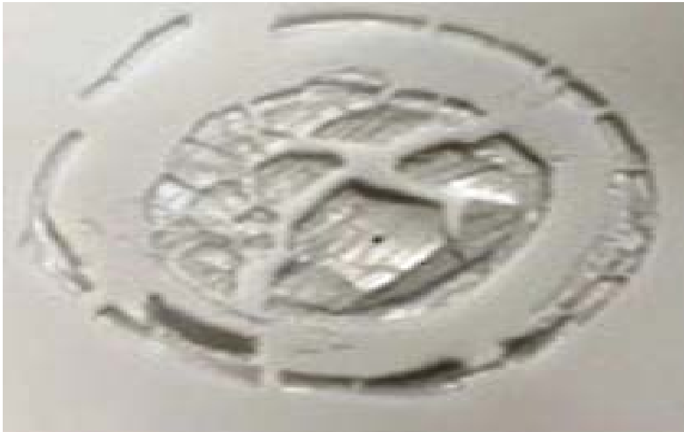
Figure 4.14. 3d-printed YSZ disk with cracks due to constrained sintering using water as the solvent and 3% methoxy cellulose as the binder.
