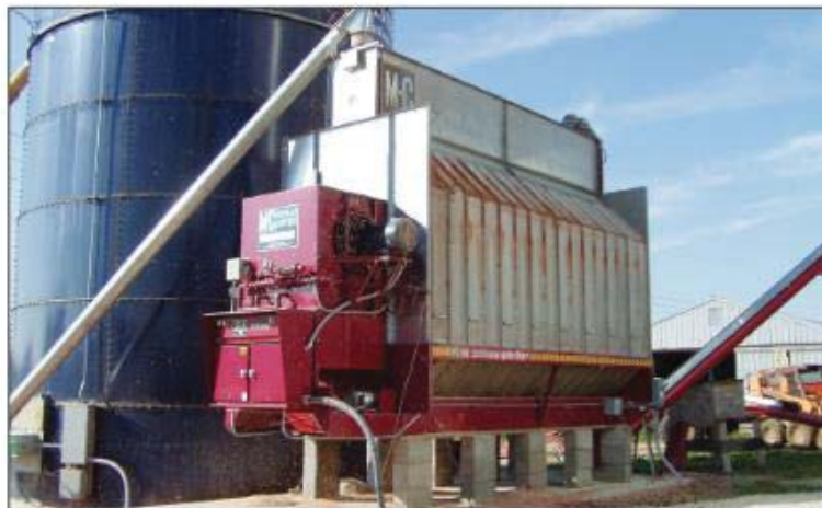
Figure 1.2-2: Typical Horizontal Cross-Flow Grain Dryer (Wehrspann, 1998)
