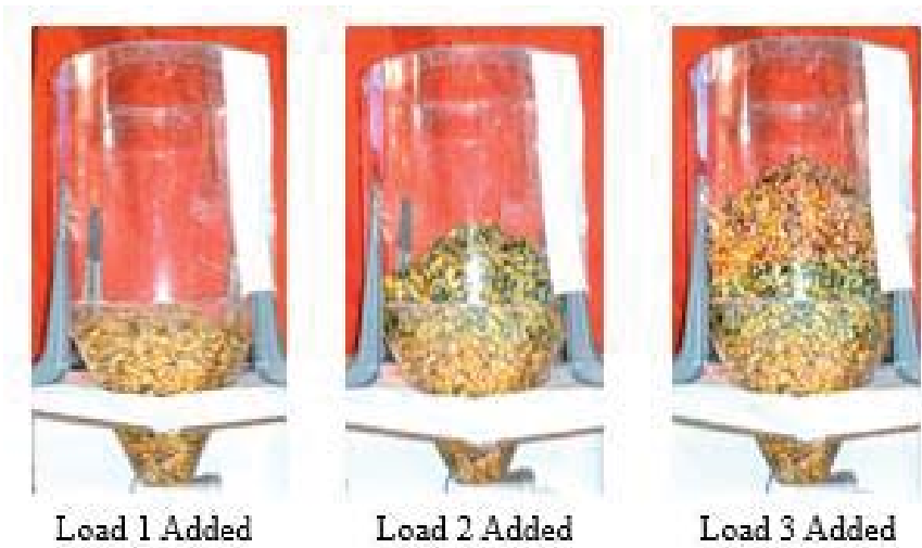
Figure 2.4-3: Filling the Test Setup Wet Bin During the Dye Test
