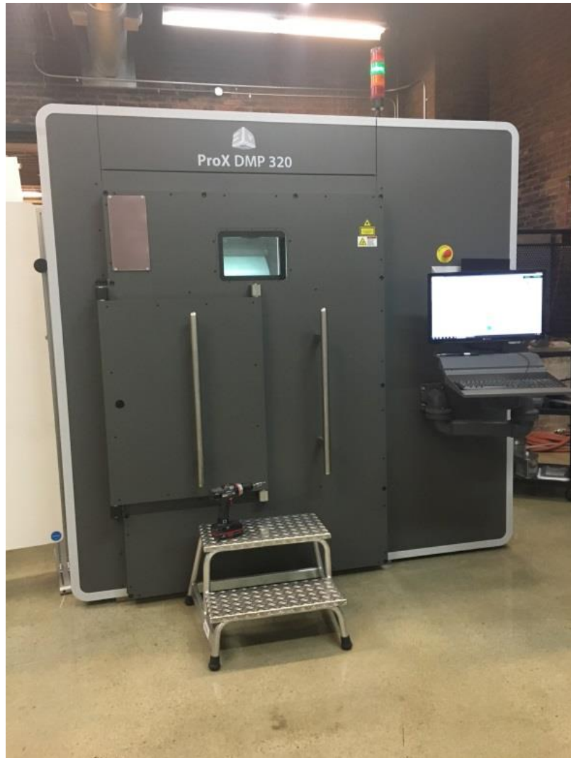
Figure 2.2: Selective laser melting machine used for printing of Inconel 718 parts.
