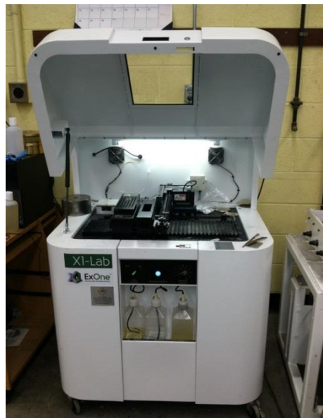
Figure 2.7: Binder-jetting 3D printer at YSU.
