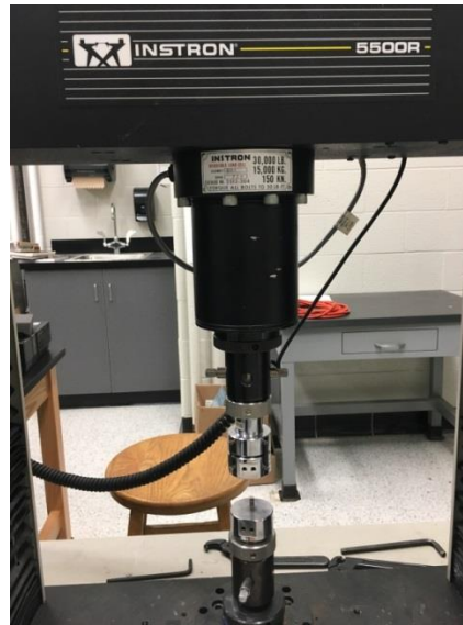
Figure 2.9: Instron machine used for compressive testing.
