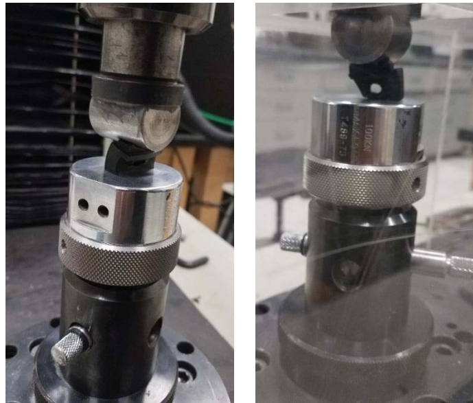
Figure 2-7 Loading of the left and right shoes
