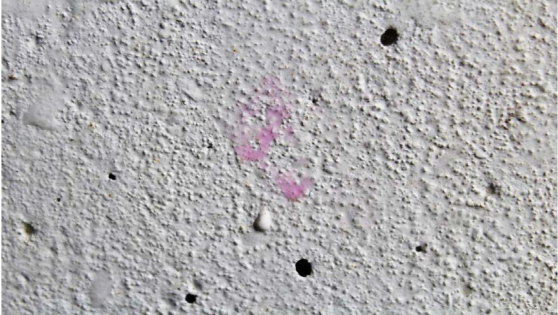
Figure 3-4: Absence of carbonation indicated as the surface becomes pink.
