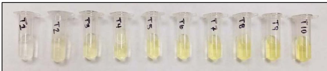
Figure 3-19: Samples collected from continuous production of oNP by immobilized BglX. The samples were retained for analysis at 405 nm.
