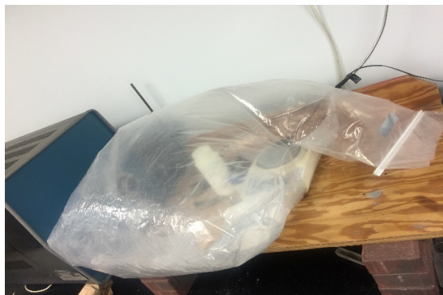
Figure 3.1. A polyethylene glove bag used for solid starting materials and product preparations.
