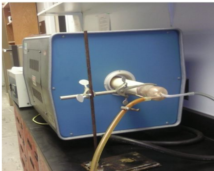
Figure 3.2. The programmable Lindberg tube furnace used for some of the high temperature reactions under argon or nitrogen gas in this work.
