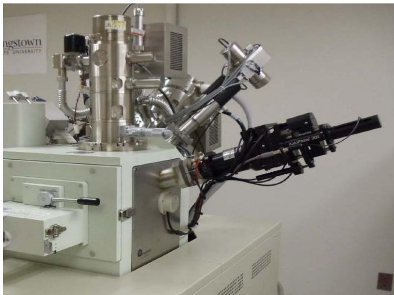
Figure 4.2. JEOL JIB-4500 Multi-beam System (SEM/FIB) used in compositional analysis of this project.
