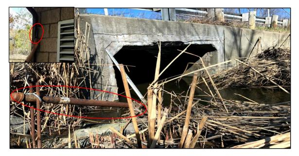
Figure 2-5: Levelogger instrument setup on the upstream side of culvert and Barologger at pump station (top left corner) on Blackbrook road
