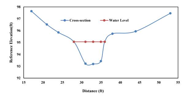
Figure 2-7: Blackbrook Creek cross-section at flow monitoring site
