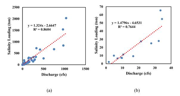
Figure 3-11: Correlation between salinity loading versus streamflow at Marsh Creek on Daily Scale (a) and Monthly Scale (b)
