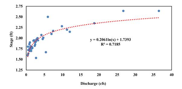
Figure 2-9: Development of Stage Discharge (rating) curve at Blackbrook Creek monitoring site
