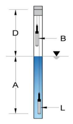
Figure 2-10: Working principle of Levelogger and Barologger
