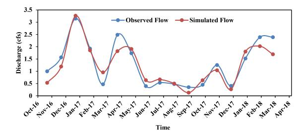
Figure 3-1: Calibrated and validated streamflow at the watershed outlet at Blackbrook Creek
