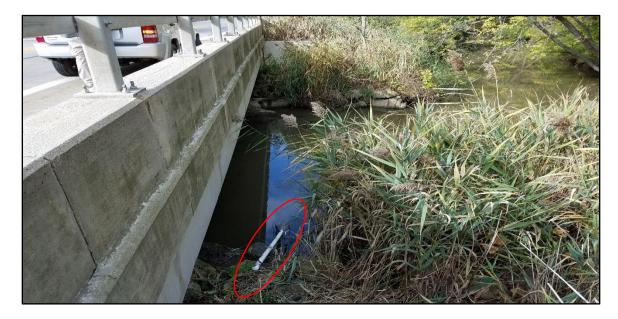
Figure 2-6: Levelogger instrument setup on the downstream side of Marsh Creek Bridge on Lake Shore Boulevard
