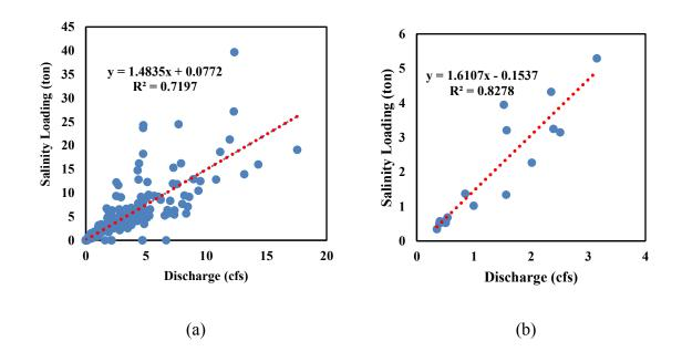
Figure 3-10: Correlation between salinity loading versus streamflow at Blackbrook Creek on Daily Scale (a) and Monthly Scale (b)
