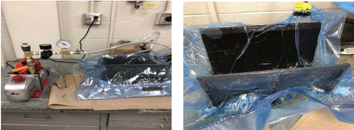
Figure 3.7: Vacuum infiltration set-up (left), and printed part during the infiltration process under vacuum (right).
