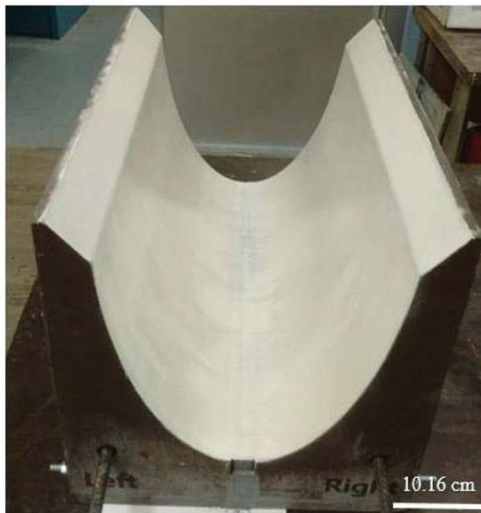
Figure 4.16: Final zirconia tooling mold infiltrated with the Freshmade3D resin #1.
