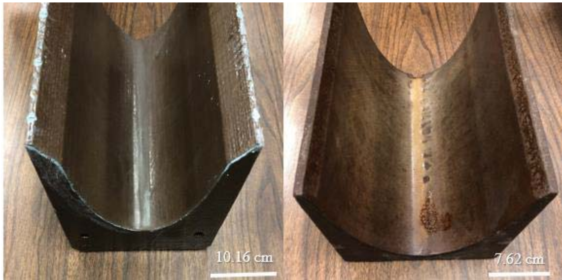
Figure 4.15: Epoxy infiltrated 3D printed ceramic tooling molds. Zirconia infiltrated with BJB (left) and silica infiltrated with BJB (right).
