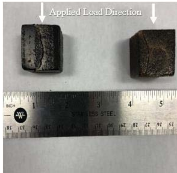
Figure 4.13: Fractured compression samples for silica infiltrated with BJB (left) and zirconia infiltrated with BJB (right).
