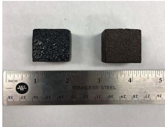
Figure 4.9: Optical micrograph of silica infiltrated with BJB resin (left), and zirconia infiltrated with BJB (right).
