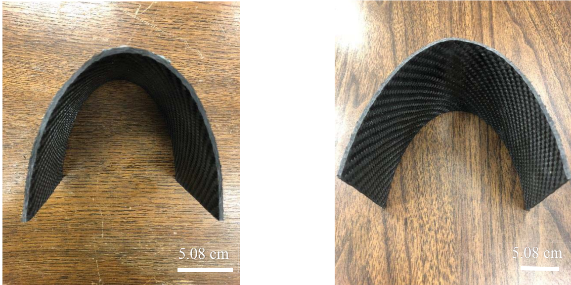
Figure 4.17: Lead edge composite parts formed on the BJB epoxy infiltrated 3D printed ceramic tooling molds.
