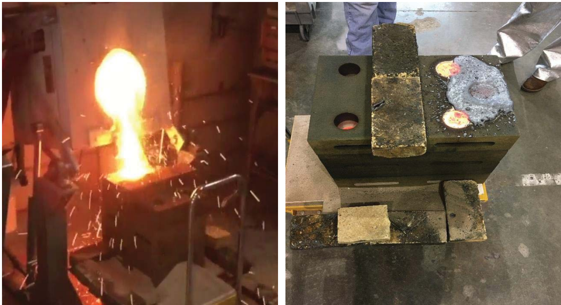
Figure 3.3: Casting process: furnace used for melting the Invar-36 (left) and the mold after the cast of Invar-36.
