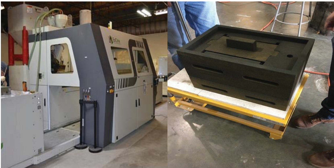
Figure 3.2: ExOne S-max binder jetting printer (left) and the assembled printed mold (right).
