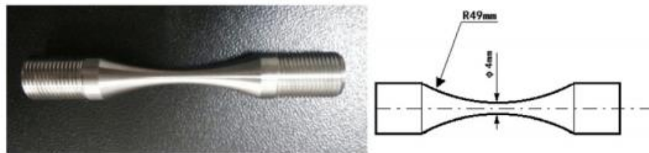
Figure 10: Fatigue Life Test Specimens
