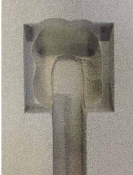
Figure 92: Milled Out Filter Base at Bottom of Sprue
