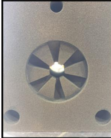
Figure 22: Inside Sand Mold of Benchmark Casting
