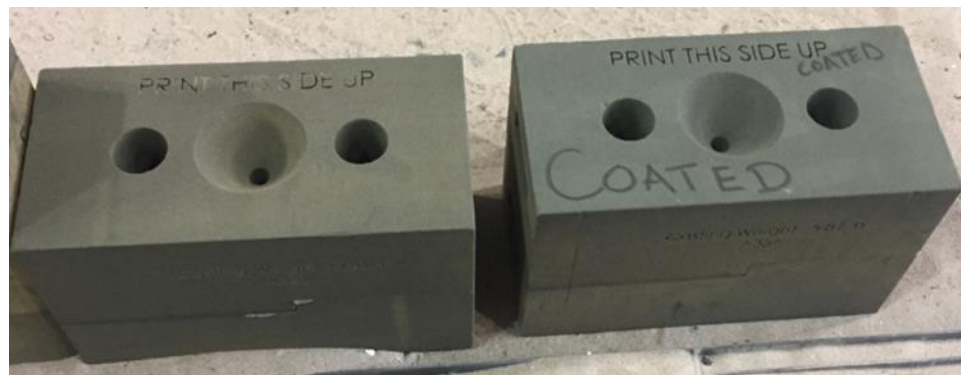
Figure 23: Sand Printed Molds
