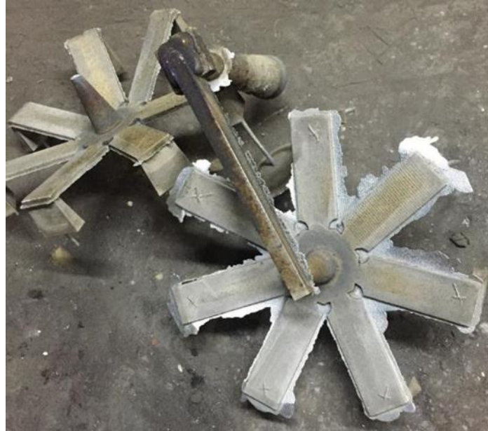
Figure 96: Casting with No Needed Assistance and Casting with Milled Out Filter Base
