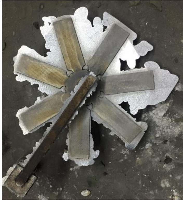
Figure 95: Casting that contained Mold with Seal
