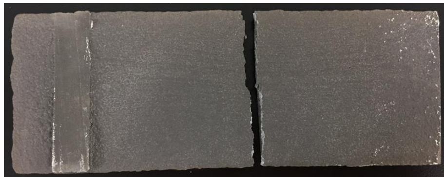
Figure 79: 0° Fatigue Test Specimen for Fractography
