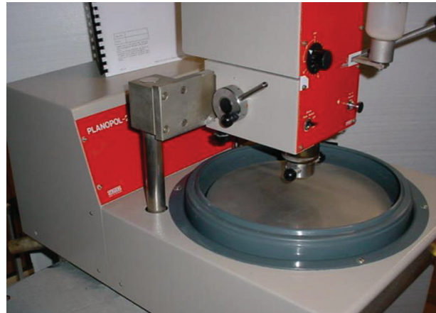
Figure 5: Struers Pedmax-2 Polisher used to polish samples
