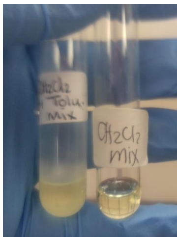
Figure 27: Crystal Growth Trial of 3b in \text{CH}_2\text{Cl}_2 and \text{CH}_2\text{Cl}_2 in Toluene Mix
