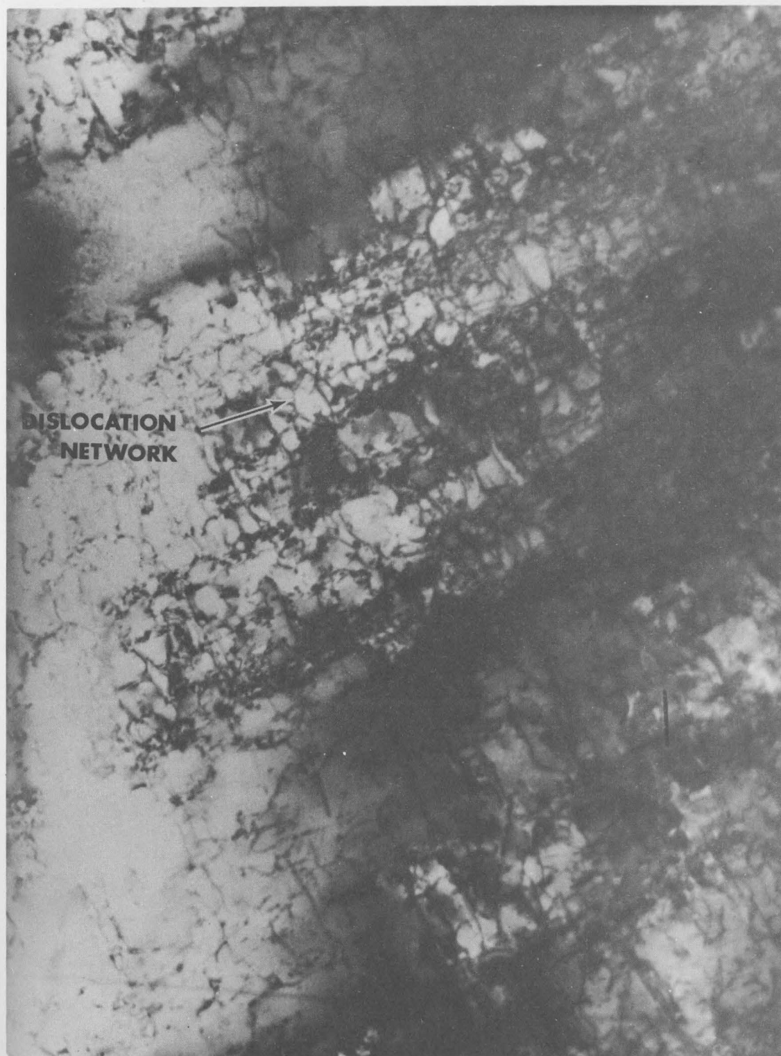
Figure 13. Transmission Electron Microscope Photomicrograph of Thinned Foil from Titanium Specimen at 26,000X Showing Dislocation Arrangements in the Plastic Zone of the Fatigue Crack.
