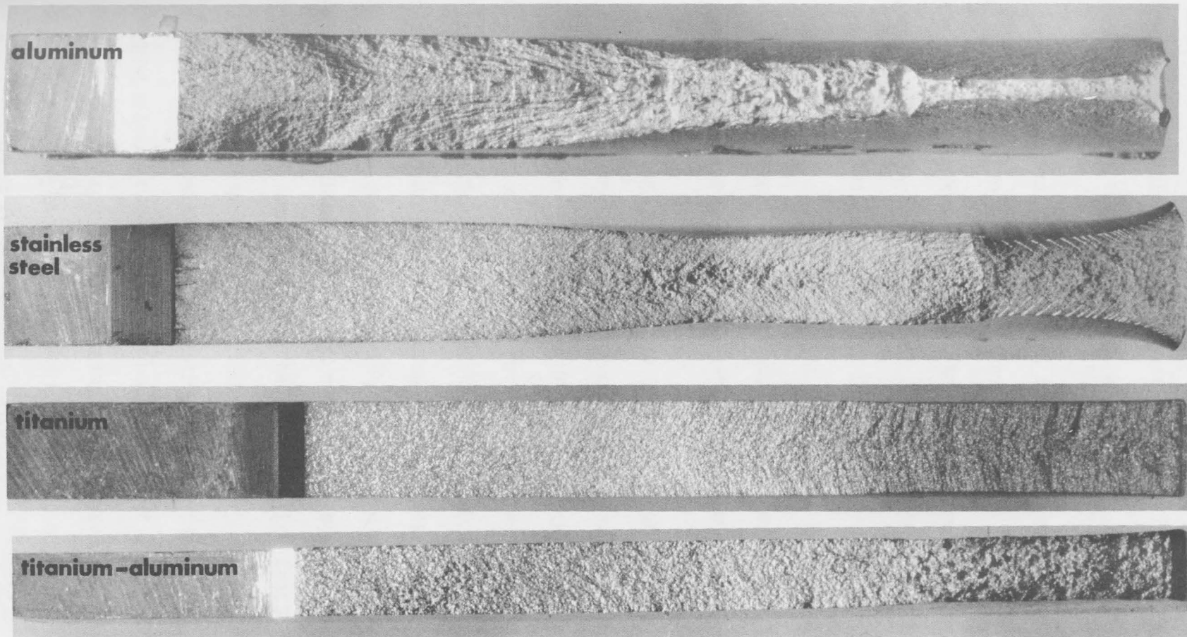
Figure 46. Optical Photomicrographs Showing Fatigue Fracture Surface Characteristics of Aluminum, Stainless Steel, Titanium, and Titanium-8% Aluminum.
