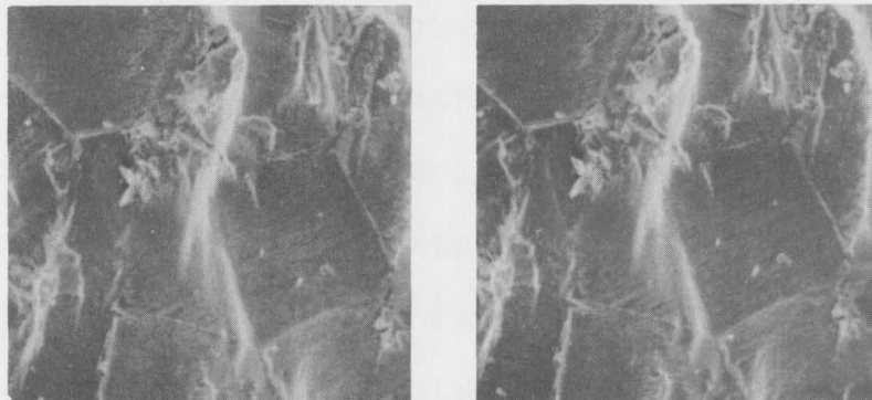
Striated Fracture (Note Grain Structure Sensitivity). High \Delta K
