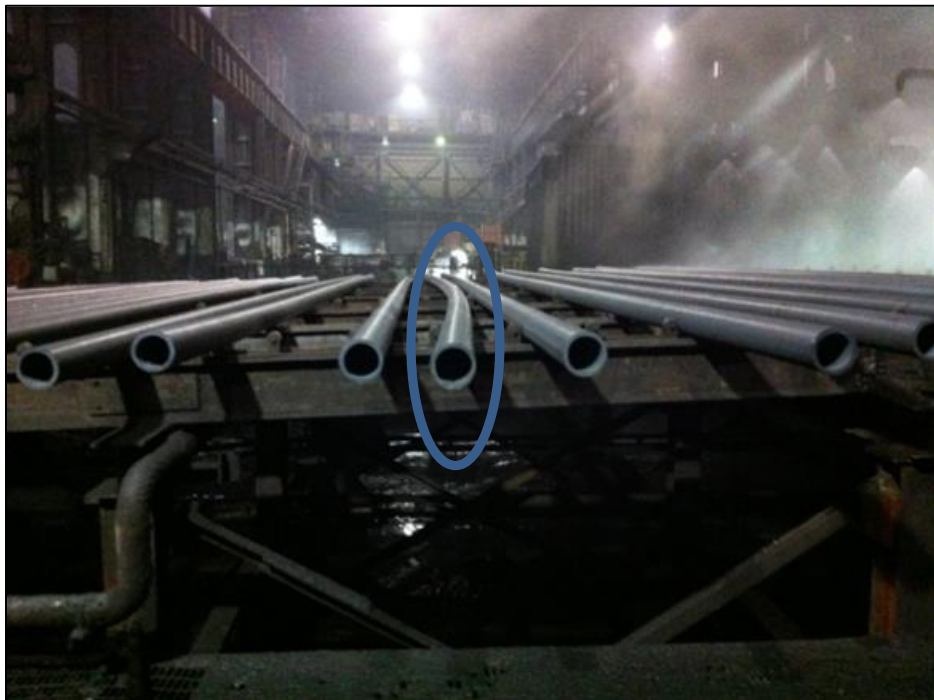
Figure 3-2: Bowed pipe during cooling process
