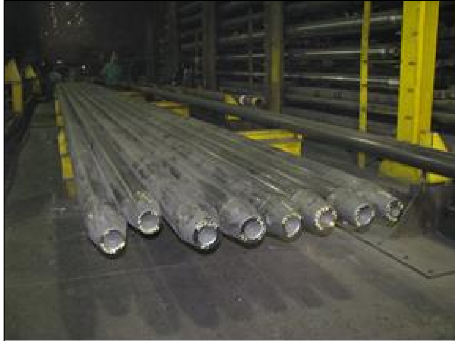
Figure 3-18: Mandrel bars laying in a rack
