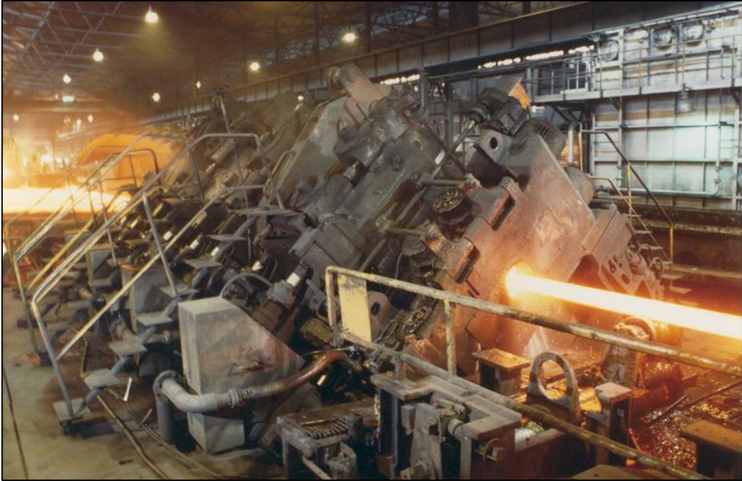
Figure 2-8: Mill stands inside of a Vallourec Facility
