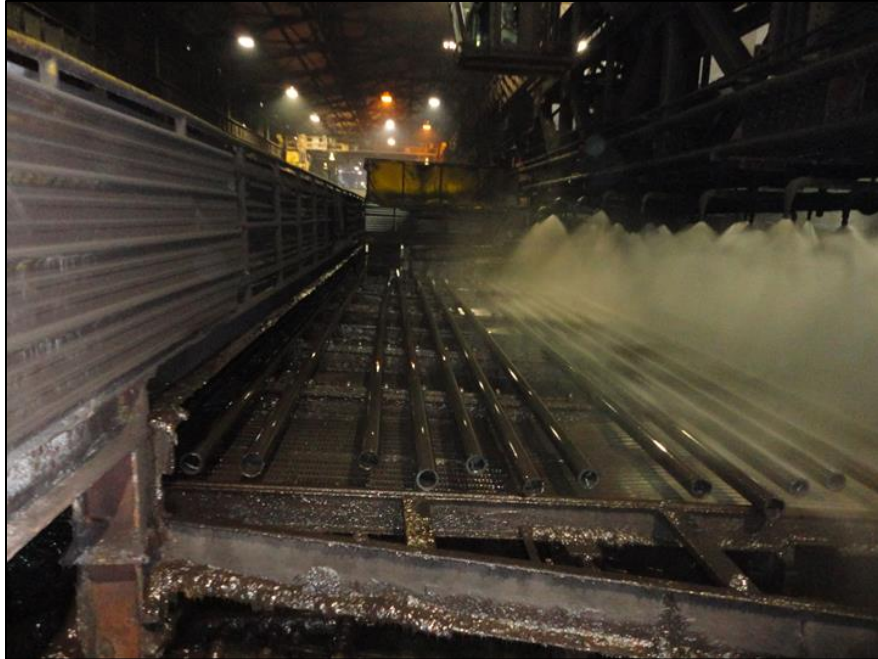
Figure 3-20: The second cooling station. Highlighting the water-cooling station
