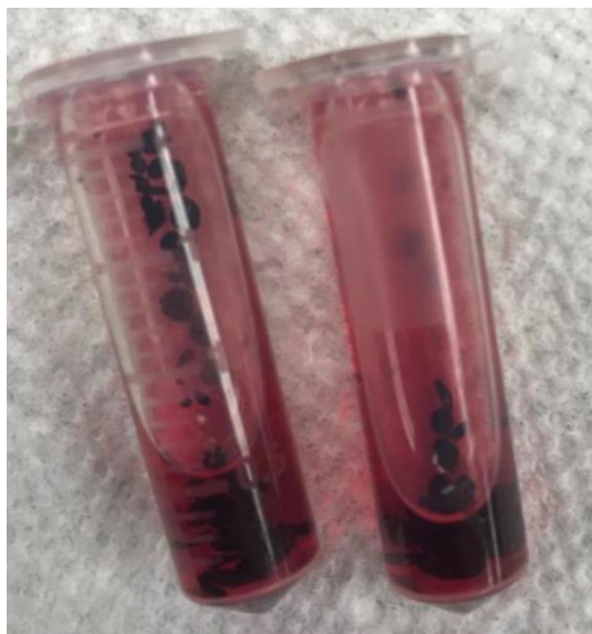
Figure 34: Hydrogen peroxide reduction in real time through: oxidation of D-glucose to D-gluconic acid and \text{H}_2\text{O}_2 coupled with oxidation of phenol/4-aminoantipyrine by \text{H}_2\text{O}_2 catalyzed by peroxidase to form pink p -quinoneimine.
