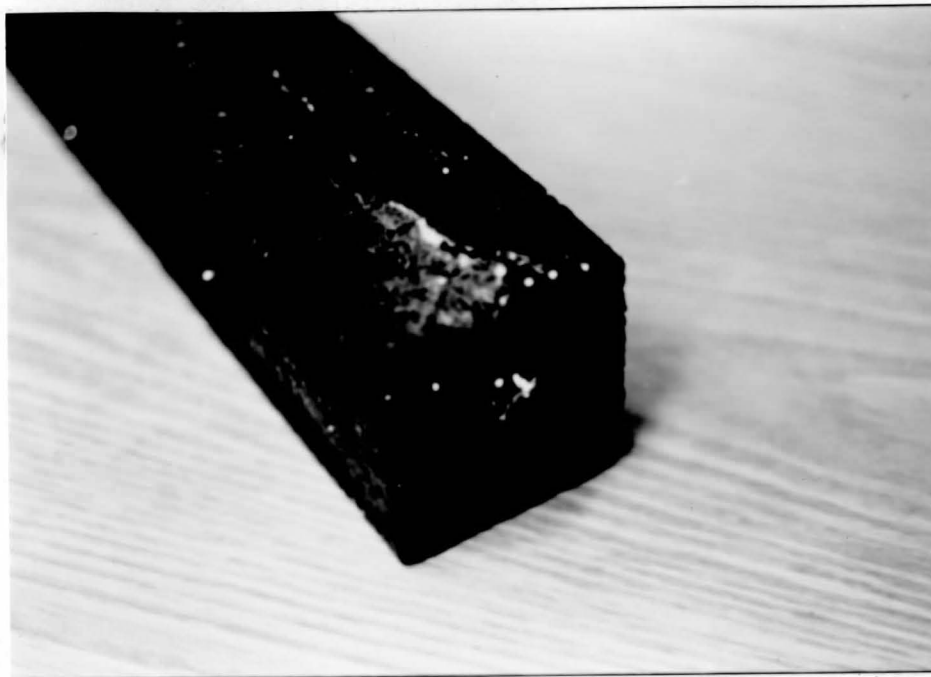
FIGURE 6.1 SPLITTING OF BITUMASTIC 300-M ON P4 AFTER 100 CYCLES
