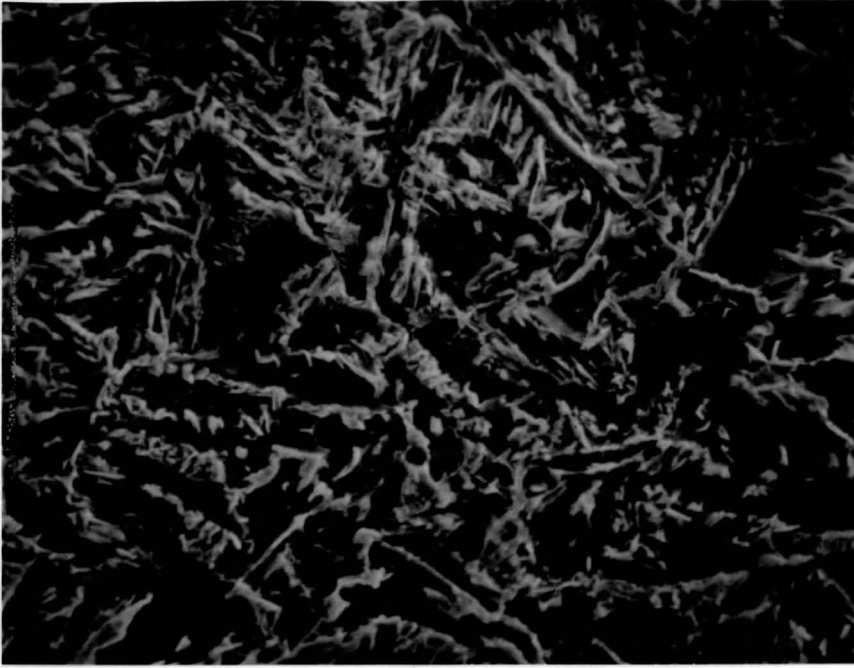
Fig. 22 -- SEM Photograph of Sample Normalized at 904°C for 5 Minutes (2000x)
