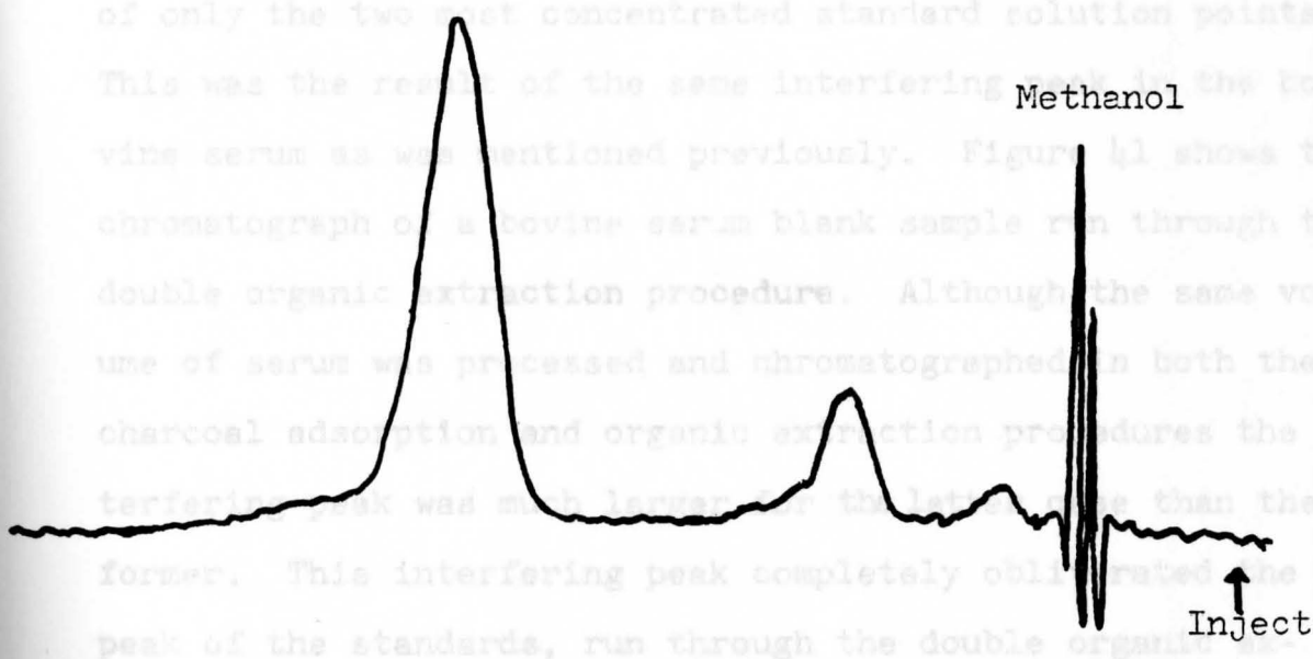
Fig. 38. -- Chromatogram for bovine serum blank (with internal standard), Charcoal Adsorption. Moving phase: pH 6.1 and acetonitrile to buffer volume ratio of 1:11. Recorder span 0.25 absorbance units full-scale.
