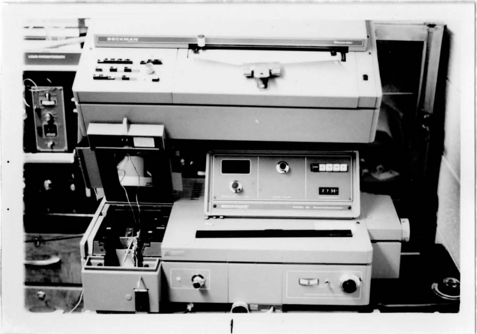
Fig. 4. -- The flow cell assembly and cradle installed in the spectrophotometer detector's sample compartment.
