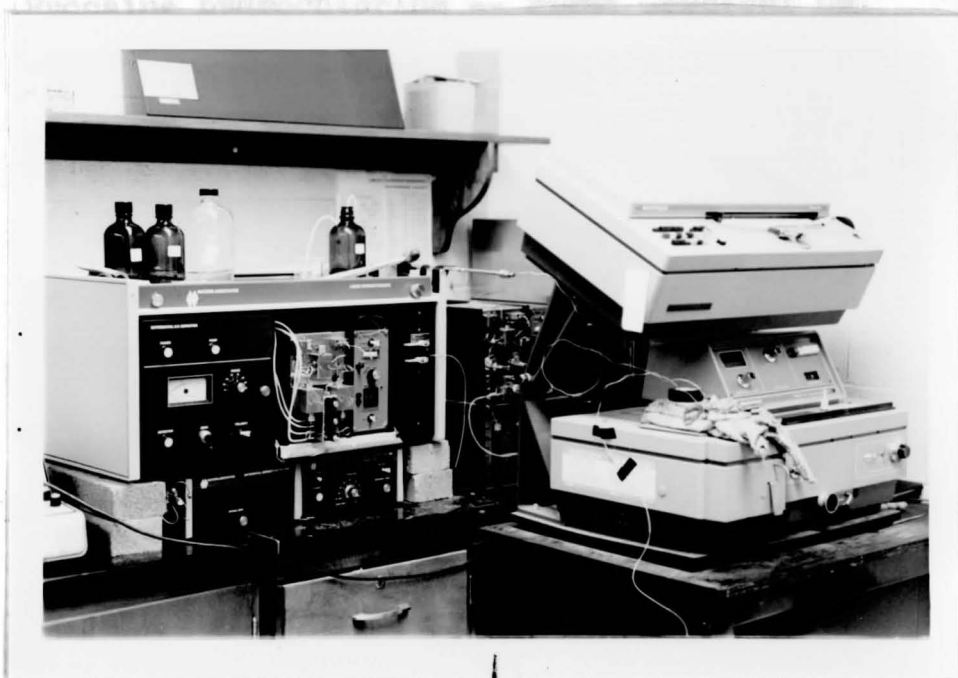
Fig. 5. -- The overall HPLC and Spectrophotometer arrangement. The HPLC is shown to the left and the spectrophotometer to the right. Note, the HPLC column shown in the upper right hand corner of the HPLC unit.
