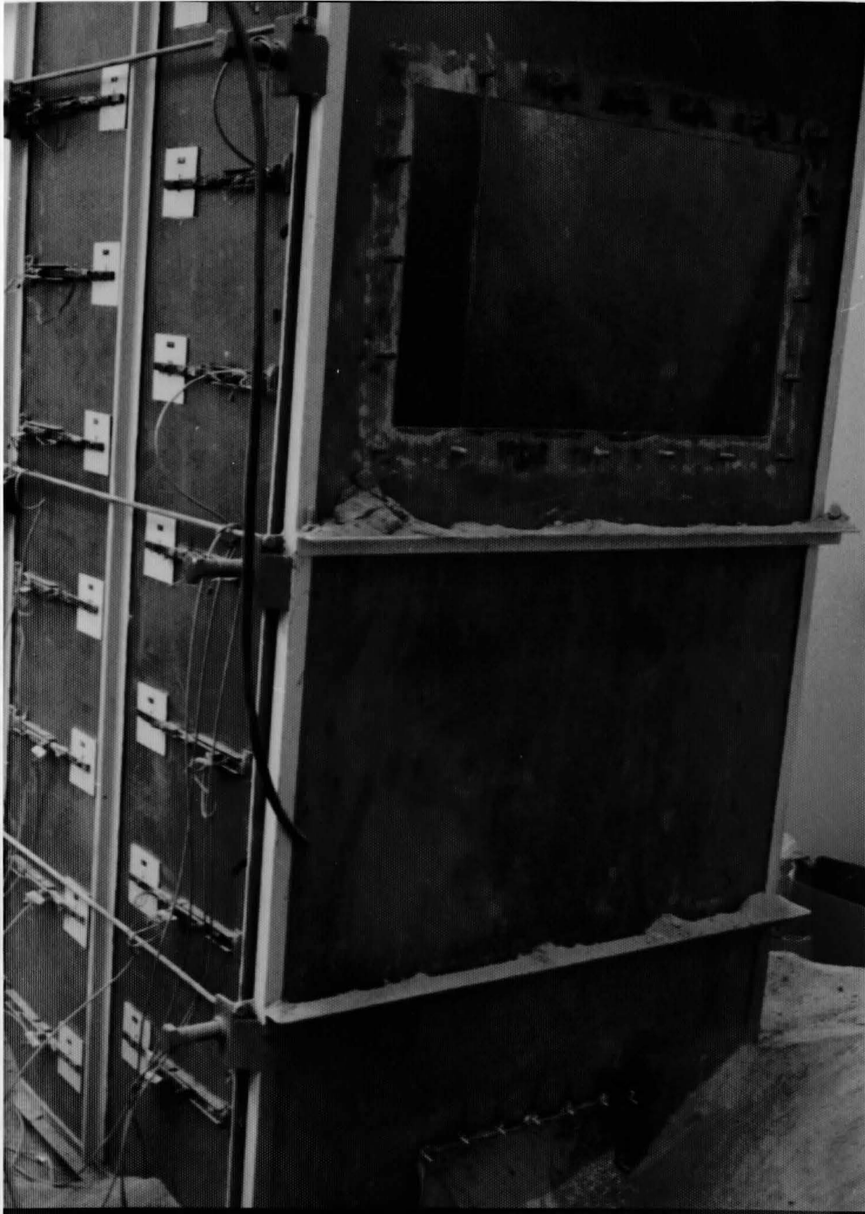
Plate No. 2 Photograph of two trap doors at the side of the steel tank to facilitate loading and unloading.
