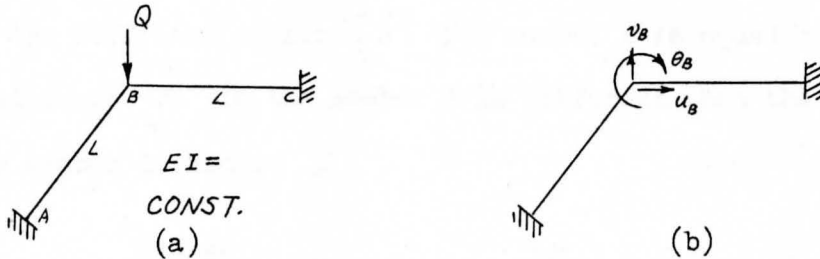
Fig. 4-8 Frame Load & Node Displacements for Problem No. 8
