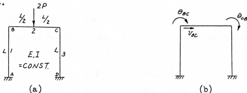
Fig. 3-7 Problem No. 3 - Frame Load & Node Displacements
