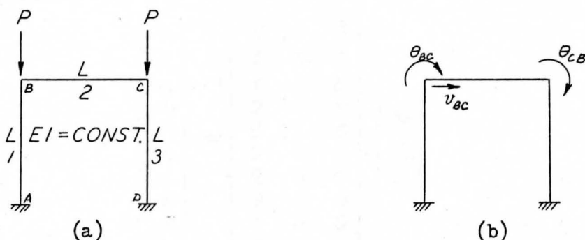
Fig. 3-1 Problem No.1- Frame Loads & Node Displacements
