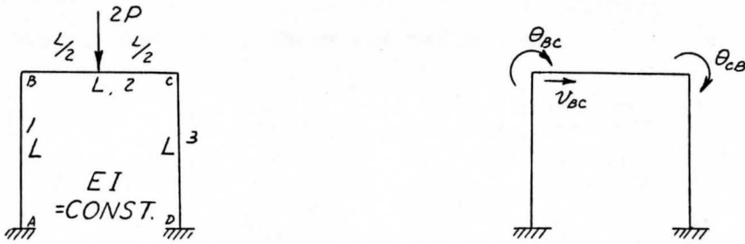
Fig. 3-11 Problem No. 4 - Member Loads & Displacements
