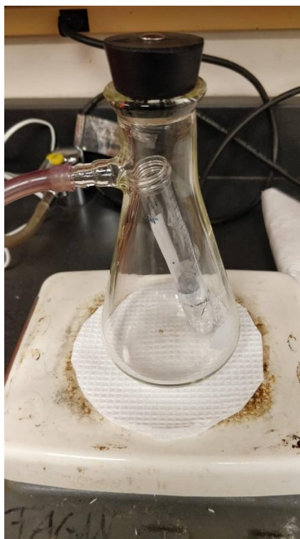
Figure 7: Vacuum Evaporator Setup. The biotinylated sample was inside a microfuge tube with the top removed and placed in a 15-mL conical tube. Aluminum foil was wrapped around the end to conduct and retain heat. A rubber stopper with a hole was trimmed and placed into the mouth of the vacuum Erlenmeyer. A wide thumb tack was used to create a vacuum seal as well as to equilibrate pressure when checking the sample for dryness.
