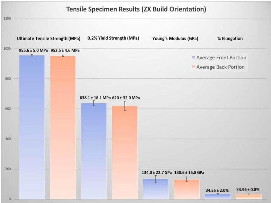
Figure 10: Tensile Specimen Results for Inconel 718 Built in the Optimized Order
