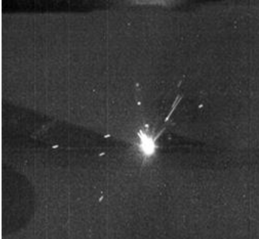
Figure 28: Spatter calving where new spatter particles have been formed and are being ejected
