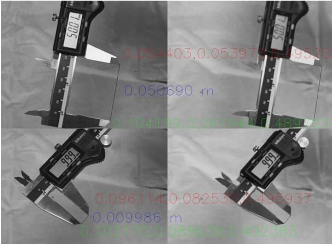
Figure 25: Stereovision quality assurance using a caliper (50.01 mm top, and 9.99 mm bottom).
