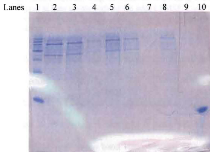
Figure 3-18: SDS-PAGE shows no protein at ~14 kDa in MMH. Lane 1 show marker, Lanes # 2-4 show cell lysate from DM3-6a, 6b, and 6c at 72 hr, Lanes # 5-8 show cell lysate from DM3-6a, 6b, and 6c at 96 hr and Lane 10 show native lysozyme.
