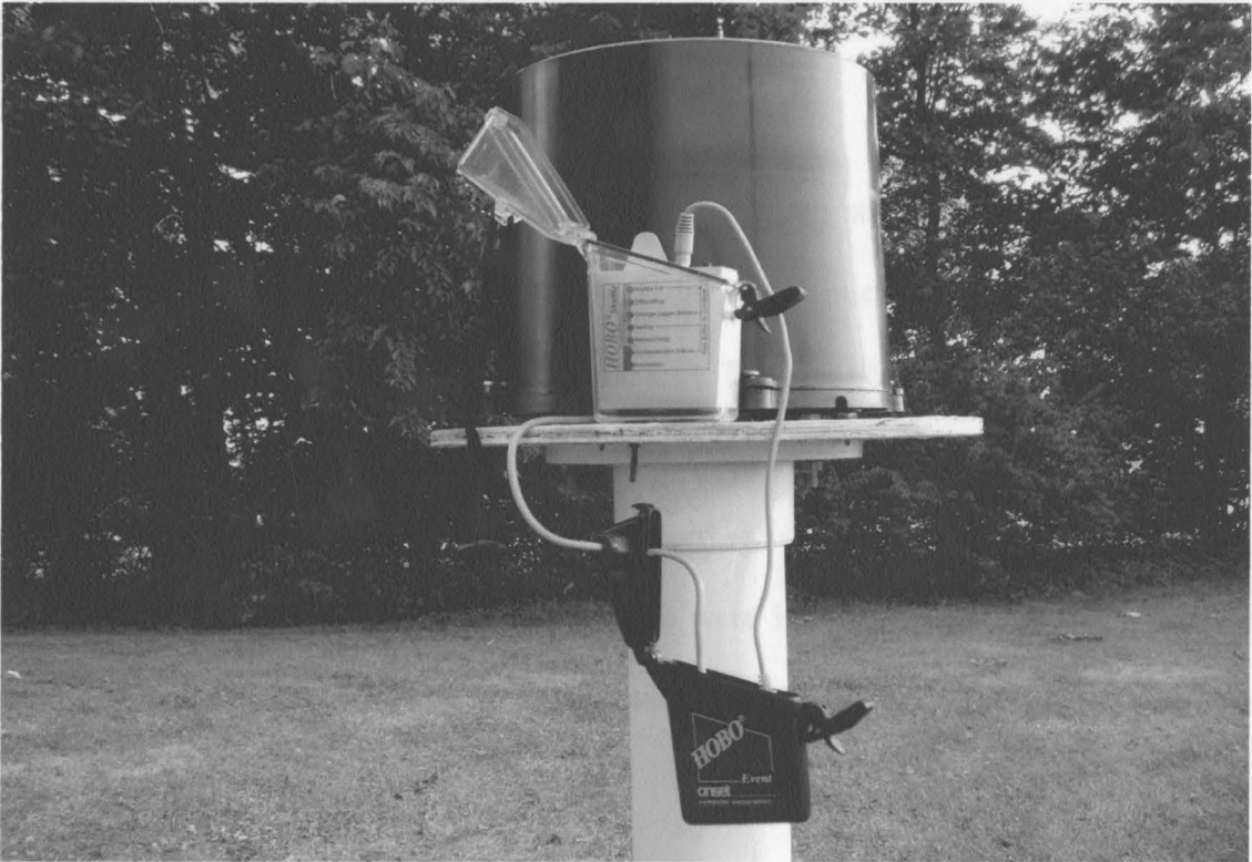
Figure 3.8 Photograph of HOBO Shuttle connected to HOBO H7 Event logger.
