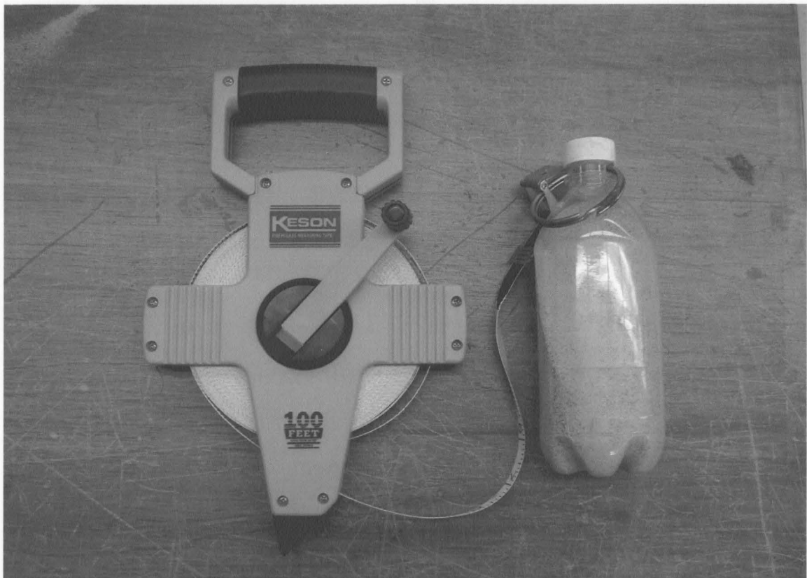
Figure 3.3 A 100 ft Surveyor's Tape Attached to 0.78 ft Bottle Filled With Sand.
