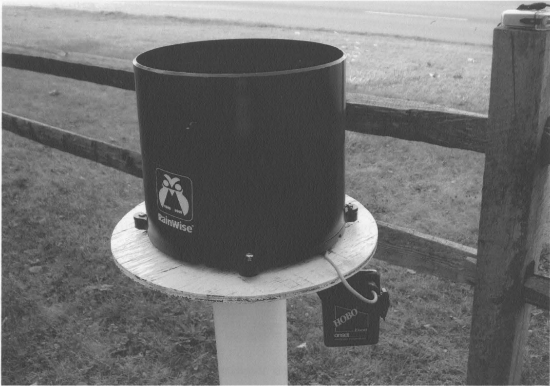
Figure 3.7 Photograph of Rain Gauge connected with a HOBO H7 Event Logger.
