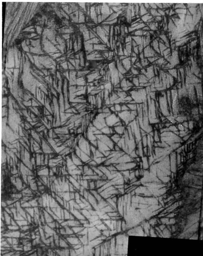
Fig. 40- Photomicrograph shows both twin traces and needle shaped transformation product in grains
