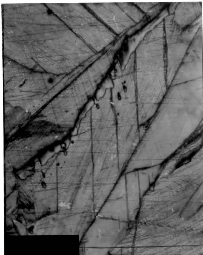
Fig. 34- Photomicrograph shows transformation product which is needle shaped Sample No: 3 Treatment: 300°C (573°K) quench Etching Reagent: Saturated solution of K_2Cr_2O_7 with 0.2% H_2SO_4 Magnification: 500X
