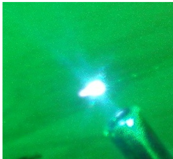
Figure 20 Laboratory produced LIBS plasma
