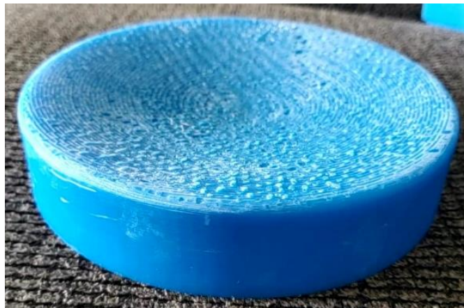
Figure 14: Draft Resin 3D printed Parabolic Disc Panel
