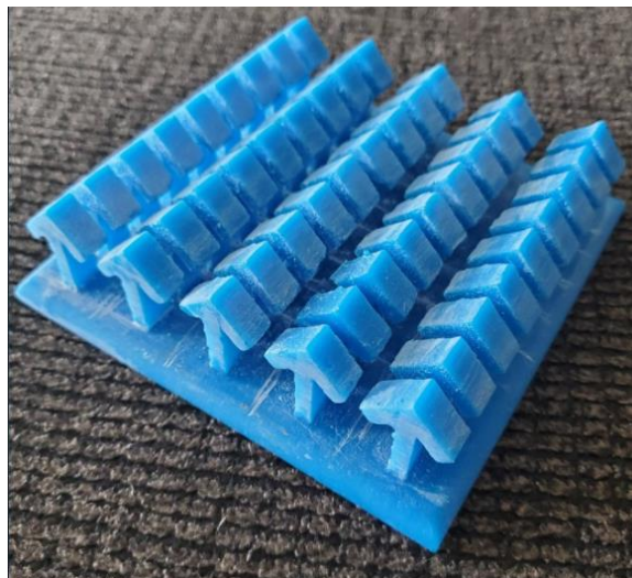
Figure 21: Draft Resin 3D printed Block Arrow Panel
