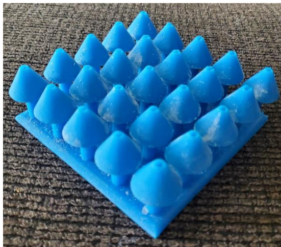
Figure 19: Draft Resin 3D printed Conical Arrow Panel
