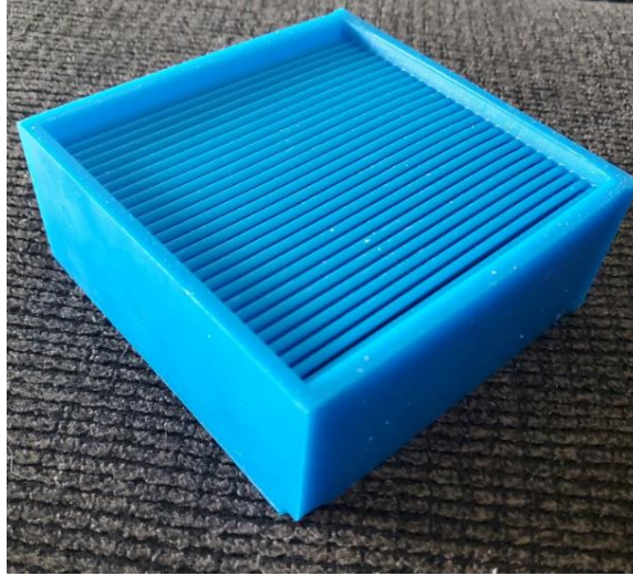
Figure 17: Draft Resin 3D printed Phononic Crystal Panel
