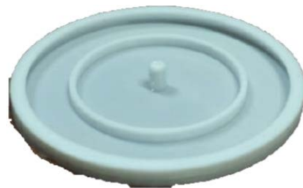
Figure 4: Printed Sample of MAM with Attached Mass Image adapted from a study by Lavie et al. [13]
