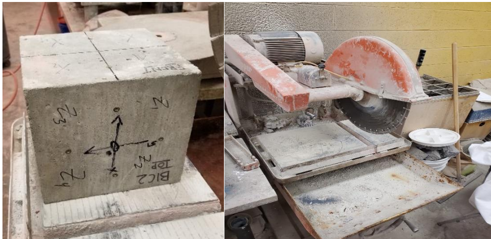
Figure 3-13 , The electrical blade used to cut the cubic specimens (pictures by Ali Qutail)
