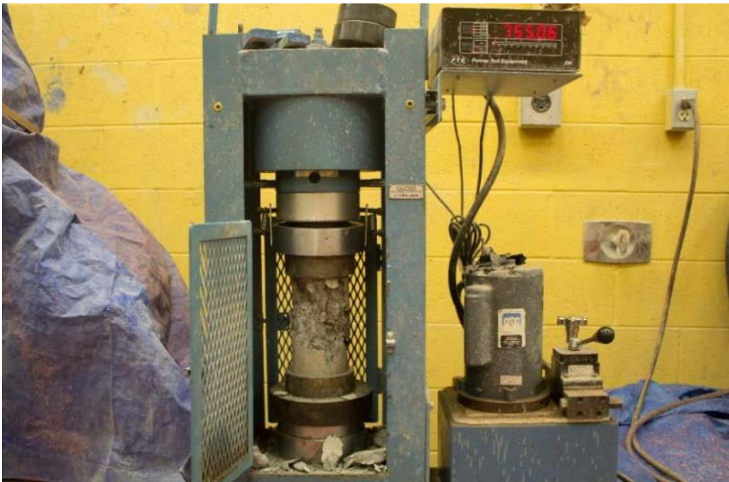
Figure 3-4 , A cylindrical specimen failed under a compressive load. (picture by Romit Thapa)
