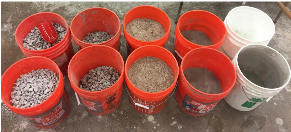
Figure 3-10 , Preparation of mix design before batching. (picture by Romit Thapa)
