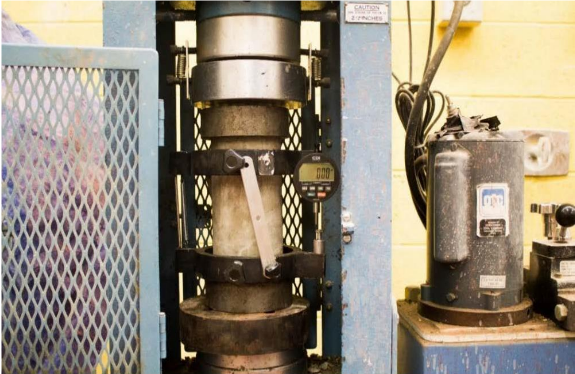
Figure 3-5, A cylindrical specimen is undergoing the modulus of elasticity test. (picture by Romit Thapa)
