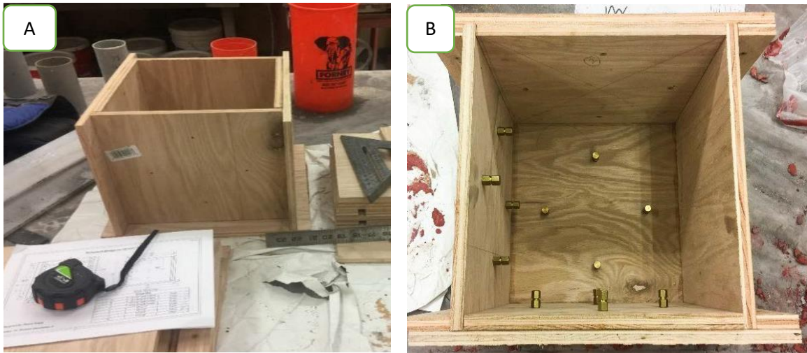
Figure 3-6, (a) A cubic ten-inch formwork. (b) Embedded expansion studs (pictures by Romit Thapa)
