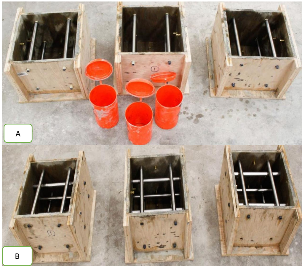
Figure 3-8 , Expansion test cubes formworks (a) Uniaxially restraint cube formwork with sheaths installed (b) Biaxially restraint cube formwork for with sheaths installed. (pictures by Romit Thapa)
