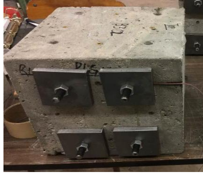
Figure 3-9 , uniaxial restraint cube after demolding and tightening the bolts (stress is applied) (picture by Romit Thapa)
