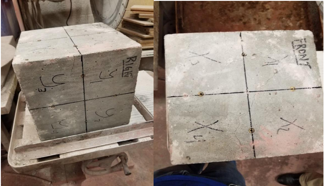
Figure 3-12 , Cubes were labeled before they were cut to 5 × 5 in cubes (pictures by Ali Qutail)
