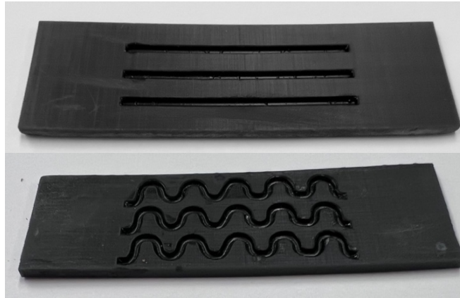
Figure 64. Printed flexible samples designed to test performance of the four inks, (top) straight line should break more than (bottom) “fractal” design which should stretch without significant breakage.
