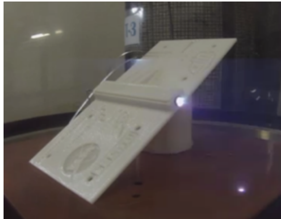
Figure 17. High voltage propulsion with embedded wires [41].
