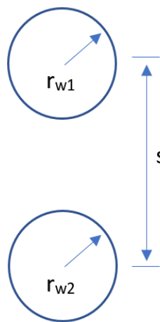
Figure 33. Dimensions used to calculate capacitance of two-wire capacitor [344].
