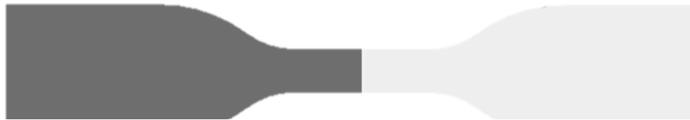
Figure 40. Example of the design of the half-tensile bars overmolded. The gray side shows one material (e.g., flexible) while the lighter one shows a second material (e.g., clear).
