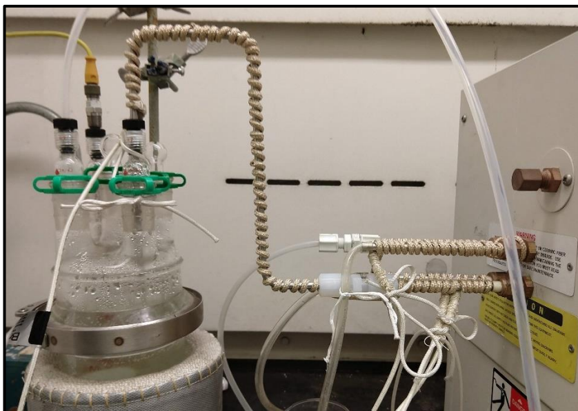
Figure 5.22: Stainless steel tubing and heating cord added to prevent condensation
