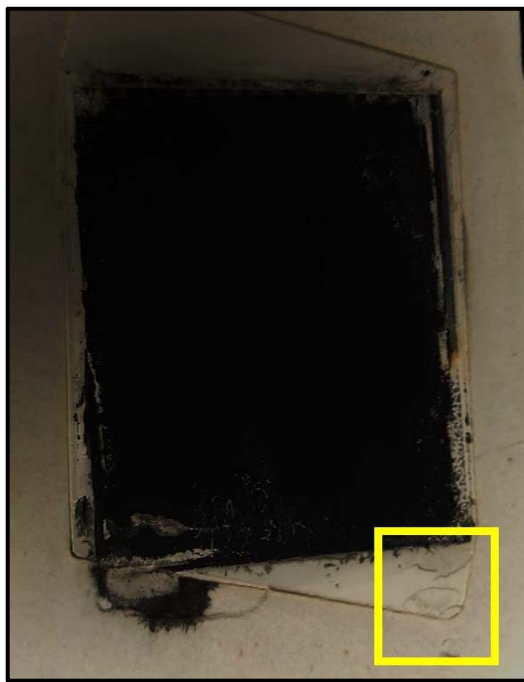
Figure 5.15: Chips in the electrolyte of Cell #3, at cathode inlet
