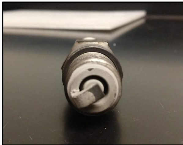
Figure 1.9: CAT 3516 reciprocating engine spark plug with a gray deposit
