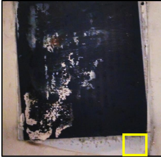
Figure 5.13: Crack at the cathode inlet area of Cell #2
