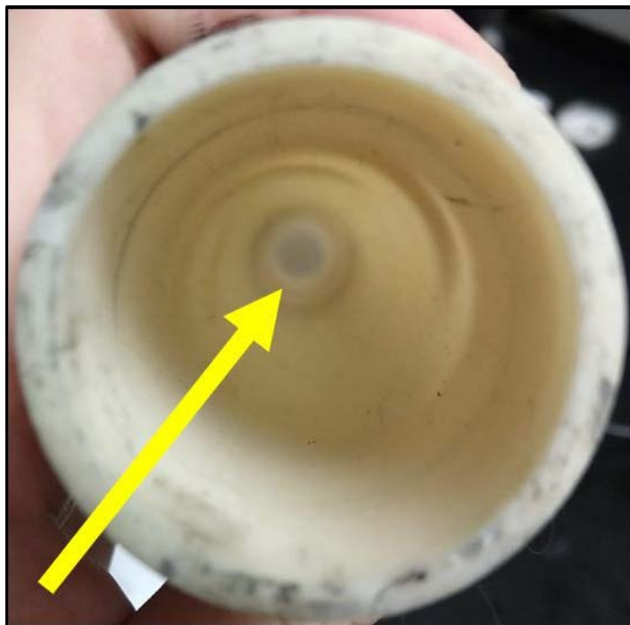
Figure 3.11: The arrow points to the white silica deposits on the inside top of the ProboStat™'s outer alumina tube.
