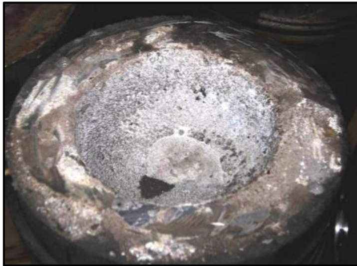
Figure 1.7: Silica buildup on the piston of a landfill gas engine 22
