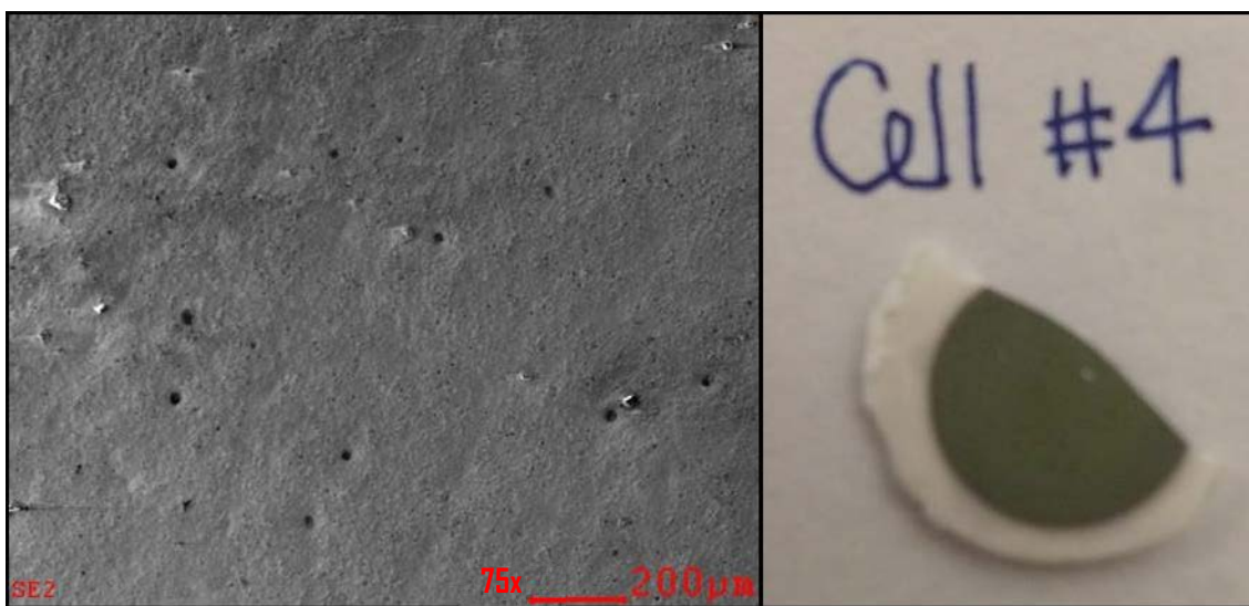
Figure 3.40: SEM image of Cell #4's anode at 75x magnification (left) and a picture showing the appearance of the cell (right)
