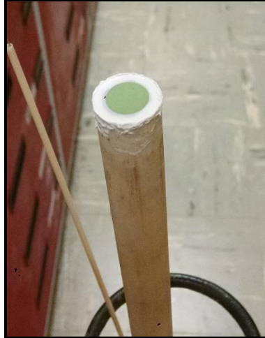
Figure 2.3: Button cell affixed to inner alumina tube of ProboStat
