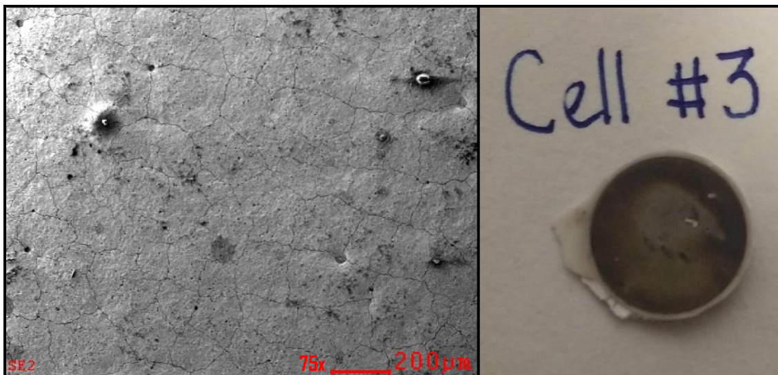
Figure 3.37: SEM image of Cell #3's anode at 75x magnification (left) and a picture showing the appearance of the cell (right)
