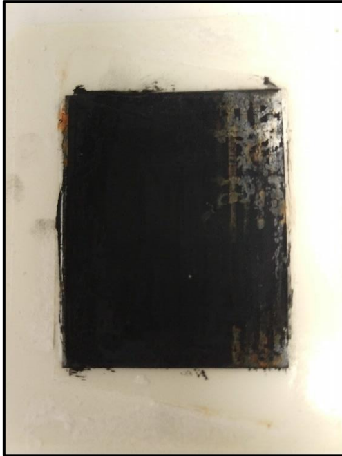
Figure 5.21: Despite a significant leak, there was no cracking in Cell #6.
