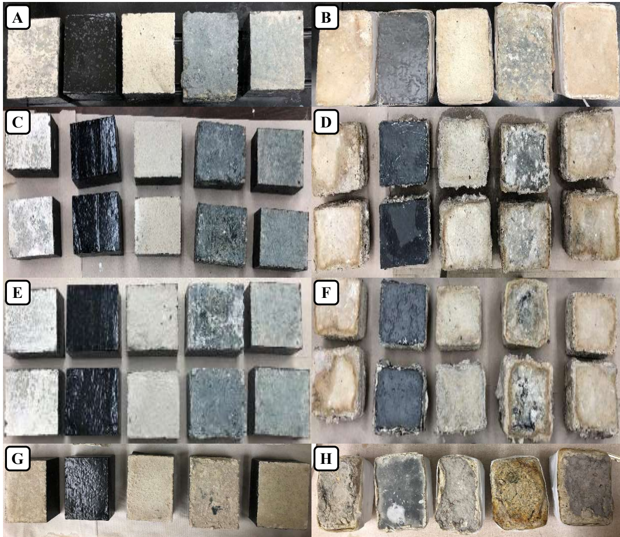
Figure 14—Progression of MICC deterioration in specimen over two years of exposure. 1 month of exposure [A-B]; 4 months of exposure [C-D]; 7 months of exposure [E-F]; 23 months of exposure [G-H]. Left column: specimen exposed to chemical corrosion; Right column: specimen exposed to biogenic corrosion. In each picture the specimens are arranged from left to right: Control, Epoxy, ARC, Biocide, NaNO 2 . (Photo(s) by Mostafa Nasr & Ramkrishna Sapkota).
