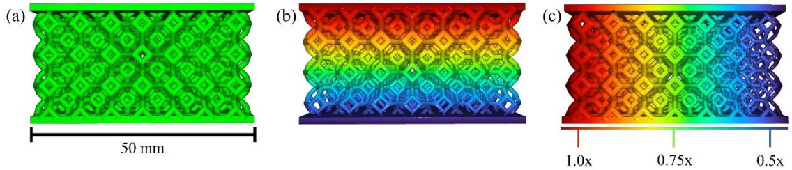
Figure 1.3: Common lattice variations; (a) non-graded, (b) vertically-graded, and (c) side-graded. Blue represents thin struts, while red represents thick struts; relative strut sizing is shown under (c).
