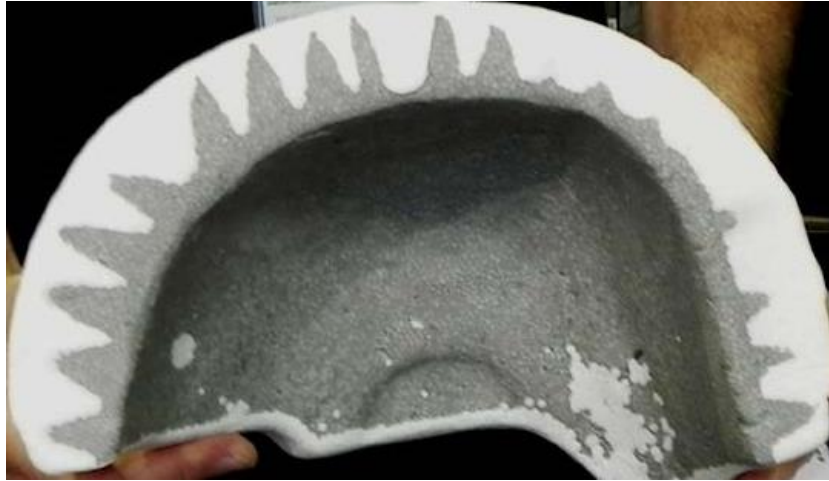
Figure 2.3: Conehead EPS foam designed with low density (grey) and high density (white) sections. The functionally-graded approach is like what is easily achievable with additively manufactured designed lattices [41].
