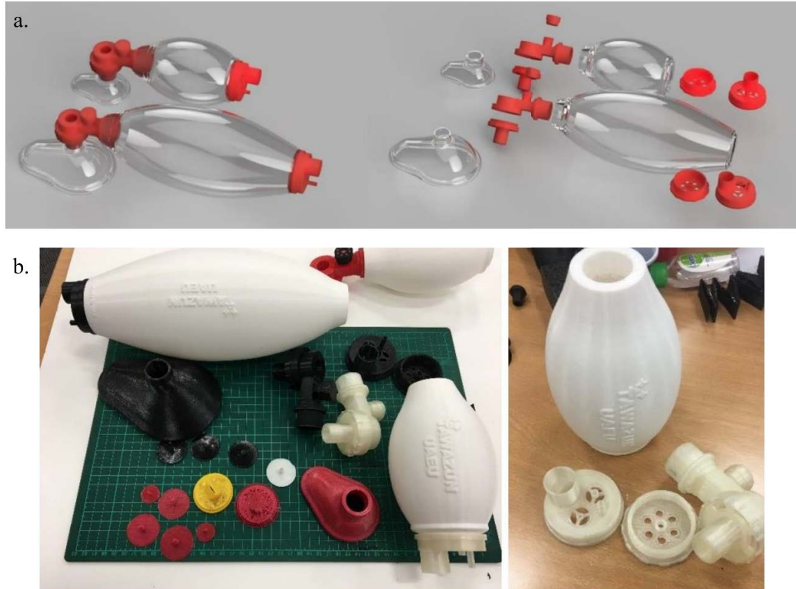
Figure 2.11: Ventilator designed by Ahmed et al. [68] in response to the COVID-19 pandemic. Photo (a) shows the different sizing possible with additive manufacturing and (b) shows the 3D printed parts from differently-colored TPU 95A. The large white vessel is the balloon for the pumping of air into a patient’s airways.
