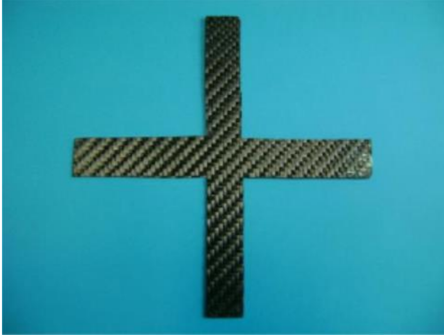
Figure 1-3: Prototype of deployable carbon fiber reinforced SMP. reinforced [13].
