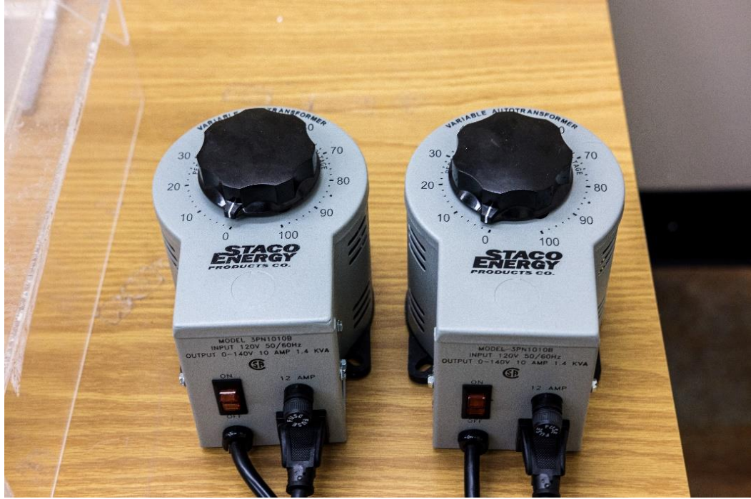
Figure 3.15: Staco Energy Variable Transformers.
