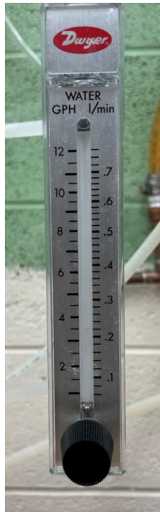
Figure 3.17: Dwyer Variable Flow Meter Used for Non-Boiling Experiment.
