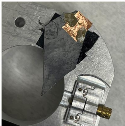
Figure 16: Sample Prepared for SEM analysis (left). SEM/FIB equipment in Electron Microscopy lab used for SEM analysis (right).
