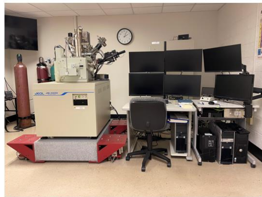
Figure 16: Sample Prepared for SEM analysis (left). SEM/FIB equipment in Electron Microscopy lab used for SEM analysis (right).
