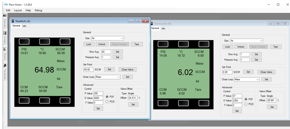
Figure 7. Flow Vision software showing sheath flow rate and atomizer flow rate
