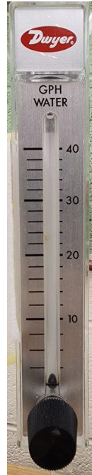
Figure 3-8: Dwyer variable flow meter.
