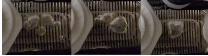
Figure 4-9: Flow-boiling visualization in MCHS configuration with single-channel manifold at \beta = 0 and average measured voltage of 41.842 V.
