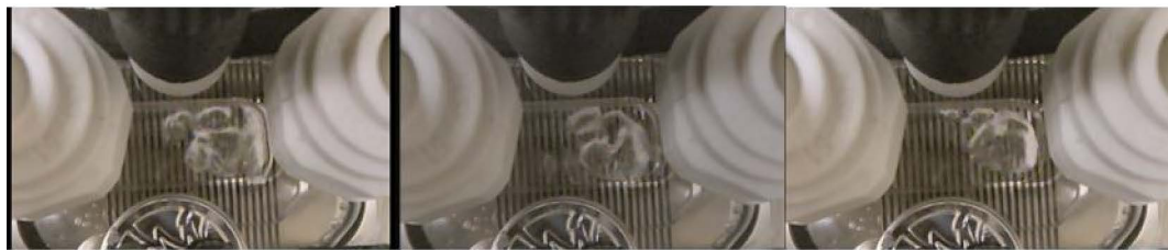
Figure 4-8: Visualization of flow boiling in single-channel manifold MCHS configuration at \beta = 0 , average voltage measured 44.785 V.
