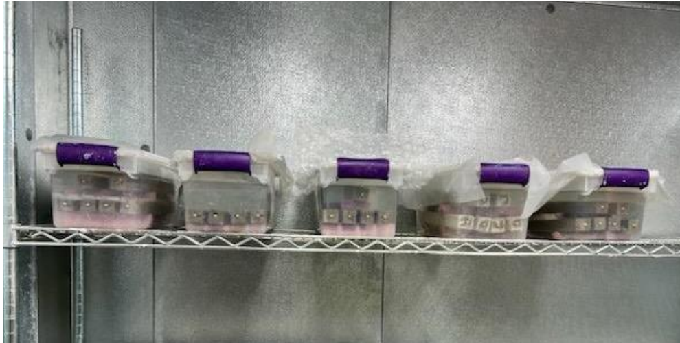
Figure 3.1 Mortar bars in containers covered and sealed to prevent evaporation and stored in an environmental chamber (Photo by Oluwafisayomi Folorunso).
