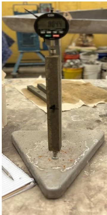
Figure 3.2 Length Check with Length Comparator (Photo by Oluwafisayomi Folorunso).
