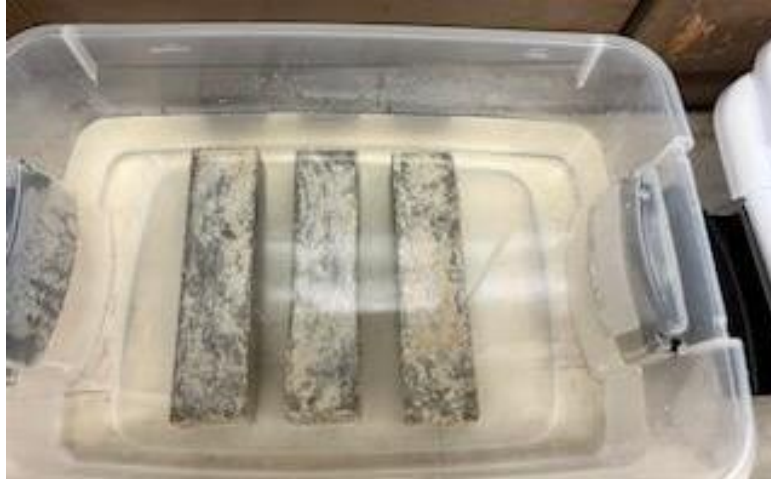
Figure 3.3 Mortar bars immersed in a sulfuric acid solution having a pH value of 2 (Photo by Oluwafisayomi Folorunso).
