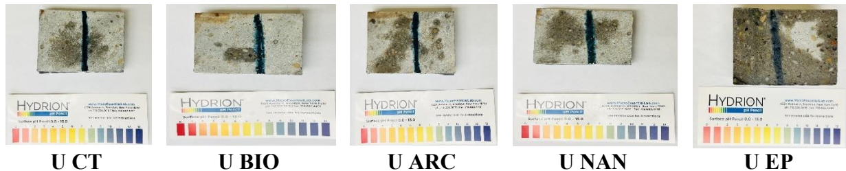
Figure 4.15 pH Imaging of concrete cross-section from control (CT), biocide (BIO), ARC, \text{NaNO}_2 (NAN), and epoxy (EP) samples exposed to chemical corrosion for two years. The pH ranged between 10 to 14 through the intact concrete (Photo by Oluwafisayomi Folorunso).
