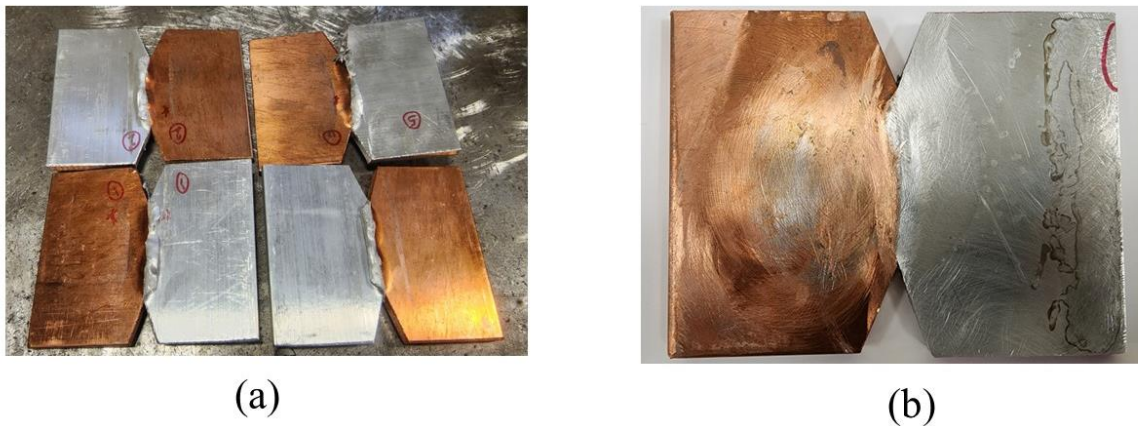
Figure 3-3: (a) Unpolished and (b) Polished Welded Sample.
