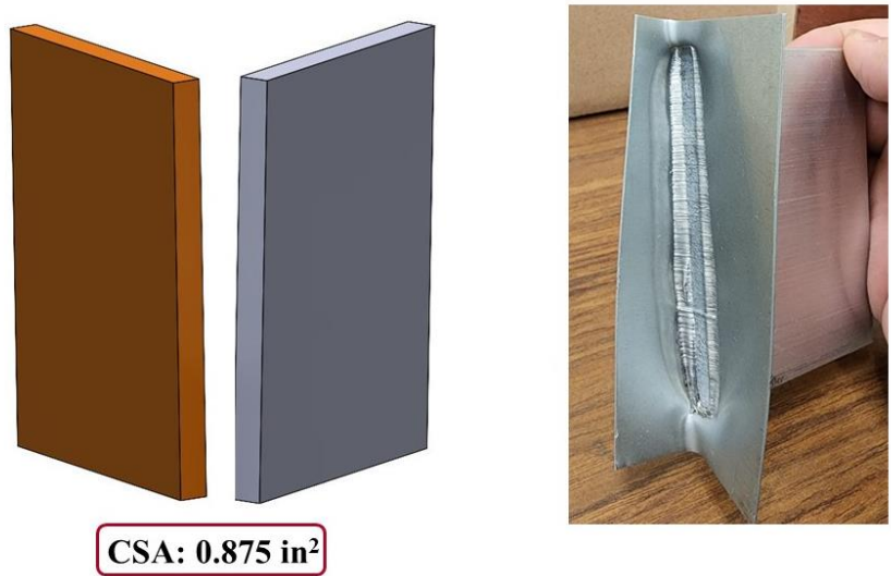
Figure 3-6: Failed welding Trial 1.
