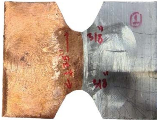
Figure 3-4: Welded sample with notch for tensile test.
