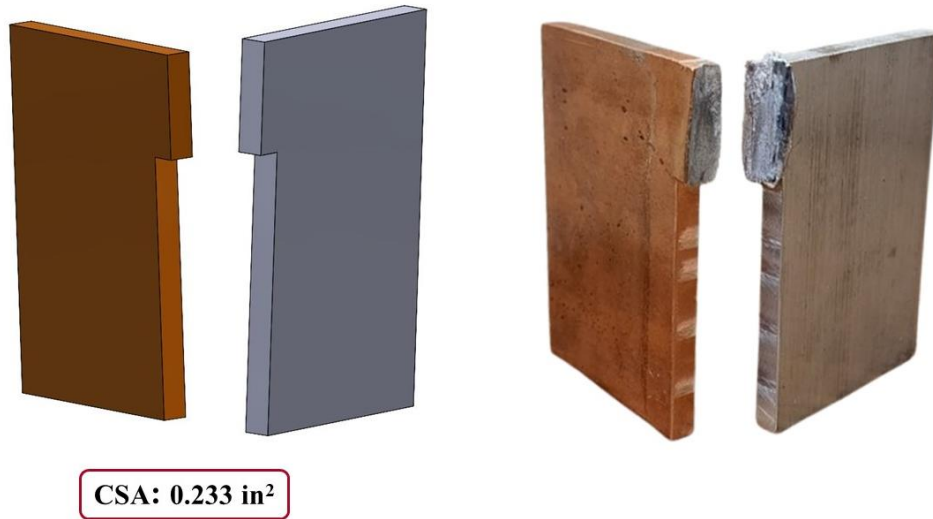
Figure 3-7: Failed Welding Trial 2.
