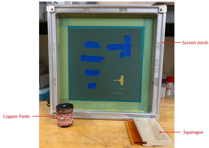
Figure 12. Screen Mesh, Squeegee and LF-350 Copper paste from Copprint.
