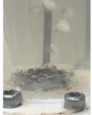
Figure 4.5: Bubble visualization of the post-wick surface in non-boiling conditions and Re = 732 .
