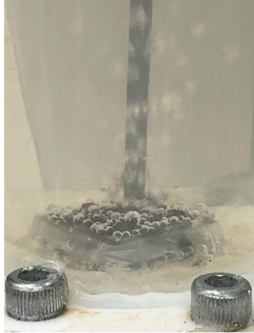
Figure 4.5: Bubble visualization of the post-wick surface in non-boiling conditions and Re = 732 .
