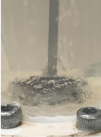
Figure 4.5: Bubble visualization of the post-wick surface in non-boiling conditions and Re = 732 .
