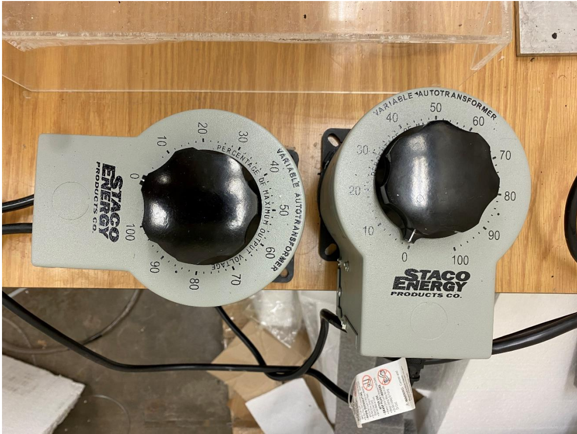
Figure 3.7: Staco Energy transformers used to power the cartridge heaters.
