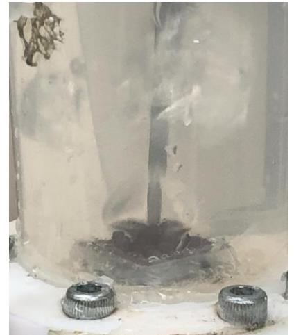
Figure 4.4: Bubble visualization of the post-wick surface in non-boiling conditions and Re = 2929 .
