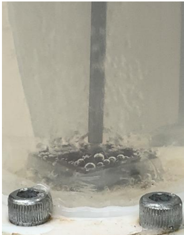
Figure 4.4: Bubble visualization of the post-wick surface in non-boiling conditions and Re = 2929 .
