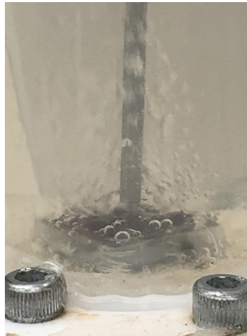
Figure 4.4: Bubble visualization of the post-wick surface in non-boiling conditions and Re = 2929 .
