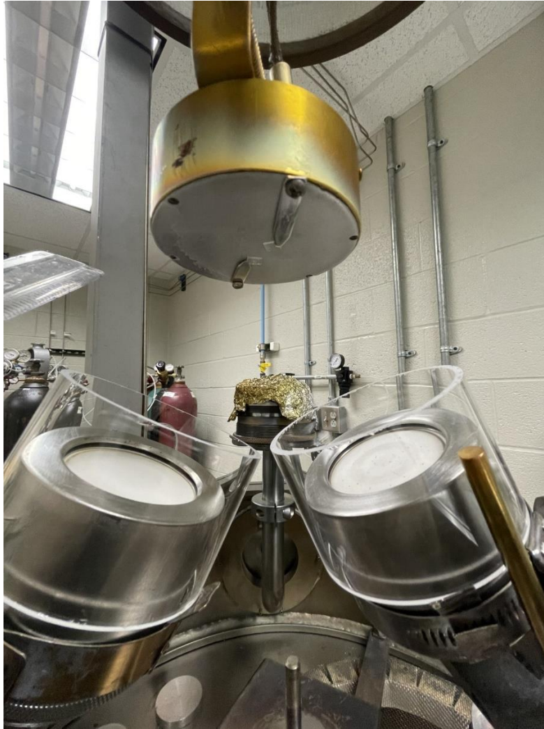
Figure 5.29 Alloys deposition setup.
