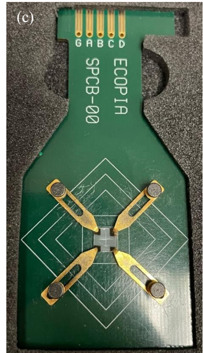
Figure 4.24 (a) ECOPIA HMS-3000 Hall effect measurement system, (b) Magnet and headboard, and (c) SPCB holder.
