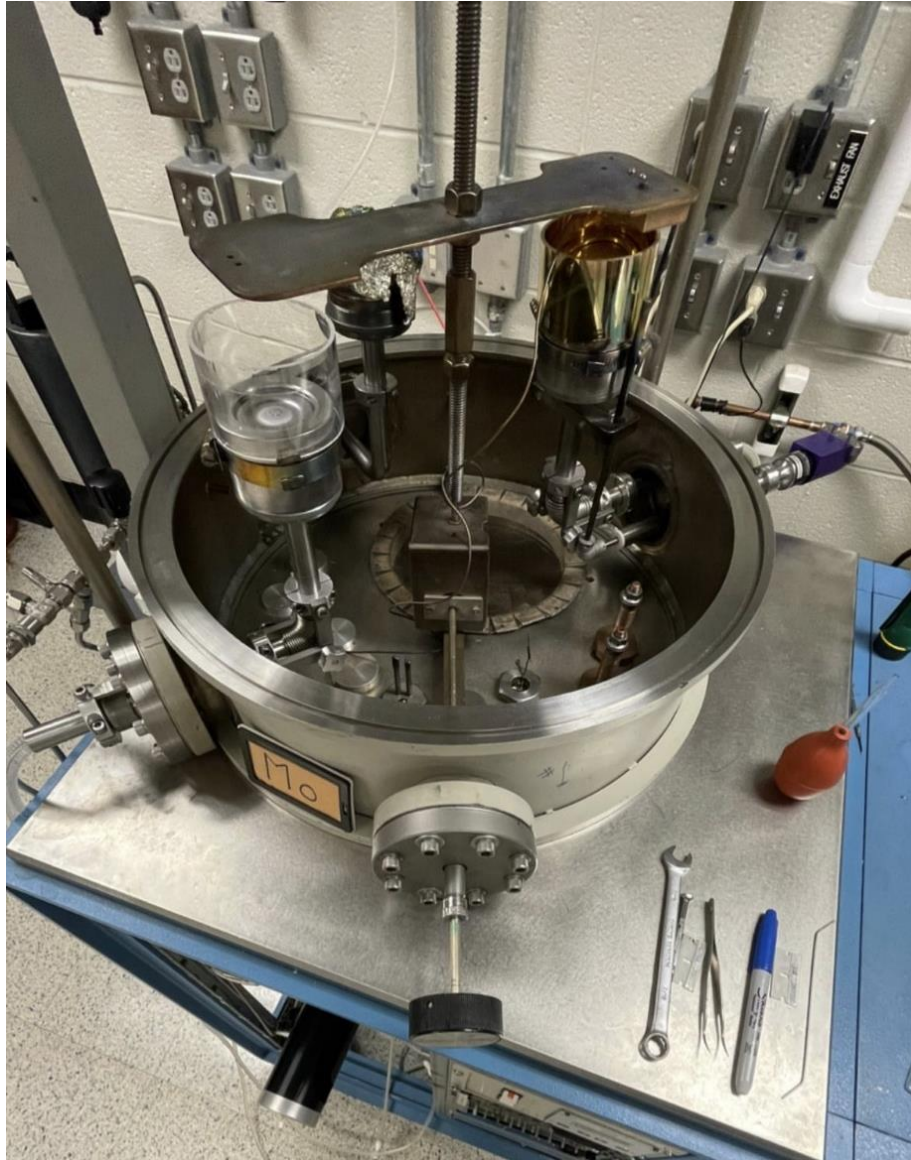
Figure 5.79 Setup for contact deposition using sputtering. The holder measures the deposition rate from which the film thickness is estimated.
