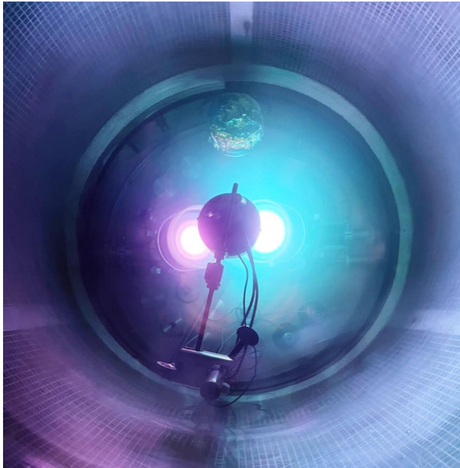
Figure 5.24 Uniform Sn-doping deposition target setup.
