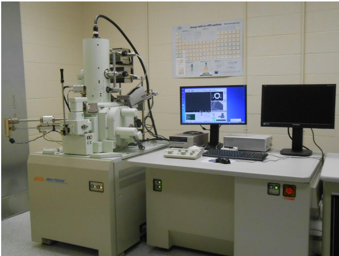
Figure 4.6 JEOL JSM-7600F scanning electron microscope.
