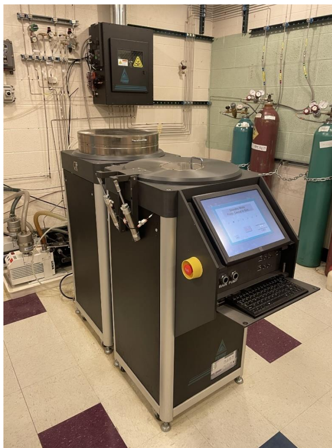
Figure 3.27 Minilock-Phantom ICP-RIE, Trion Technology.
