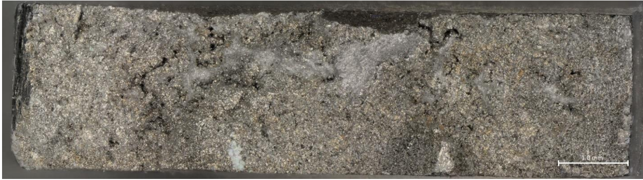
Figure 99: Top-Half Fracture of 43.5-Day Sample 6D Taken at a Magnification of 100x
