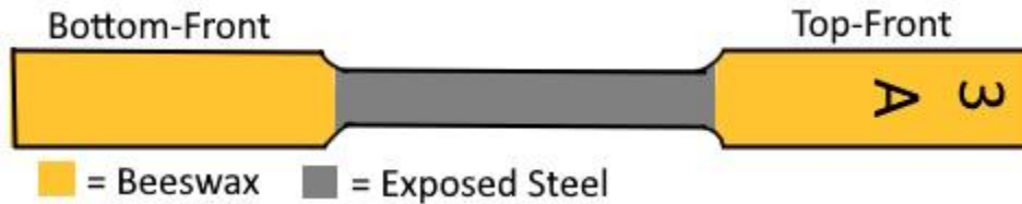
Figure 7: Example Tensile Sample with Label and Beeswax-Coverage prior to Corrosion
