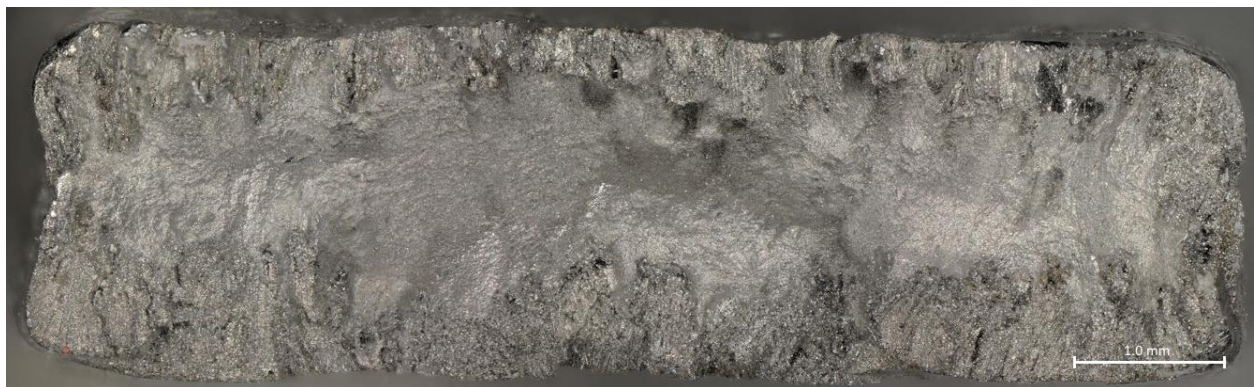
Figure 82: Top-Half Fracture of 21-Day Sample 5C Taken at a Magnification of 100x
