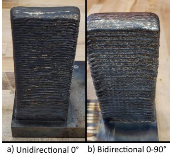
Figure 4: a) Unidirectional vs b) Bidirectional Build-Orientations Before Wire EDM
