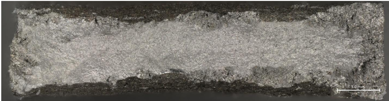
Figure 76: Top-Half Fracture of 21-Day Sample 9A Taken at a Magnification of 100x
