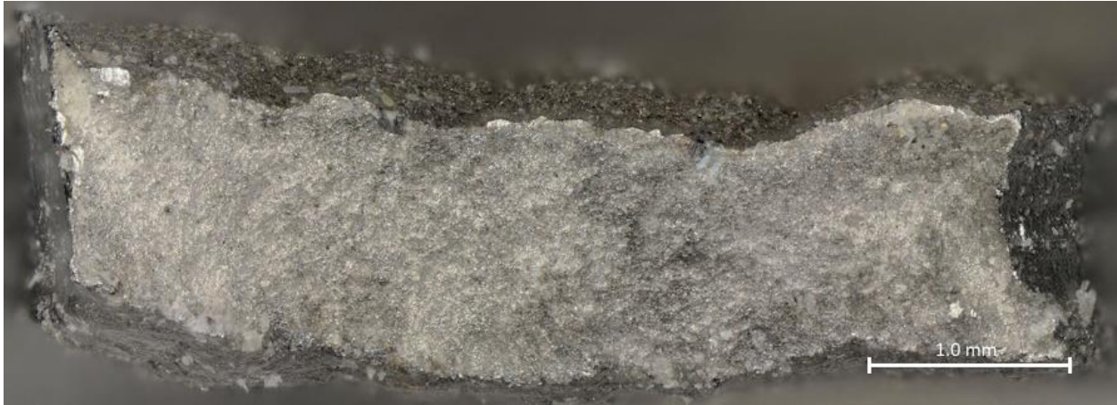
Figure 62: Top-Half Fracture of Control Sample BA Taken at 100x Magnification
