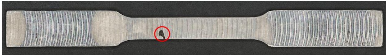
Figure 69: Optical Back Image of 1D Depicting a Surface Pit with a Red Circle
