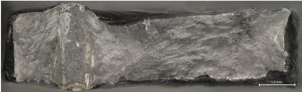
Figure 63: Top-Half Fracture of Control Sample 5B Taken at 100x Magnification
