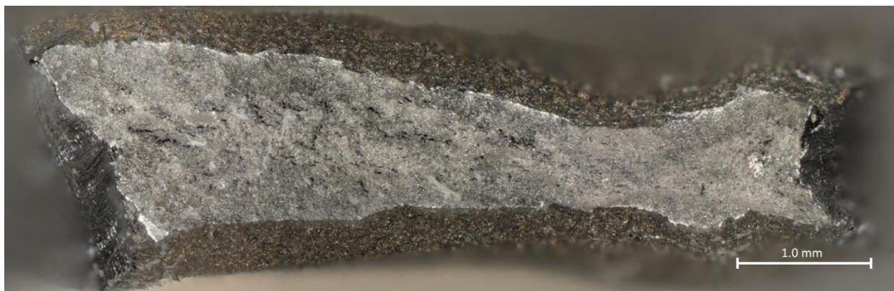
Figure 59: Top-Half Fracture of Control Sample 3A Taken at 100x Magnification
