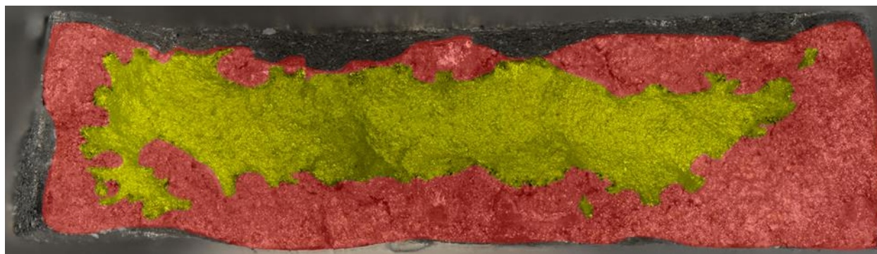
Figure 101: Fracture of 2A with the Pristine Regions Highlighted Yellow Versus the Corroded Regions Highlighted Red
