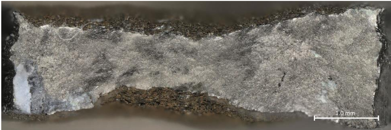
Figure 72: Top-Half Fracture of Control Sample 7D Taken at a Magnification of 100x
