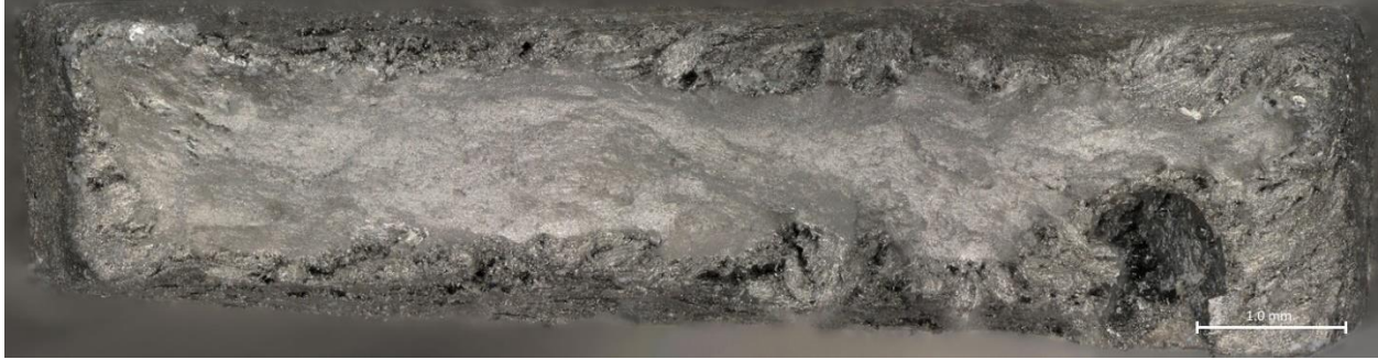
Figure 92: Top-Half Fracture of 43.5-Day Sample 9B Taken at a Magnification of 100x
