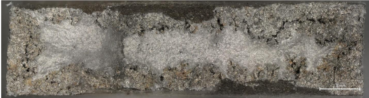
Figure 83: Top-Half Fracture of 21-Day Sample 2D Taken at a Magnification of 100x
