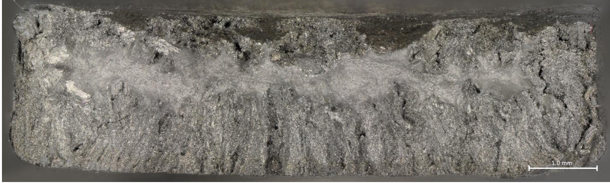
Figure 97: Top-Half Fracture of 43.5-Days Sample 8C Taken at a Magnification of 100x
