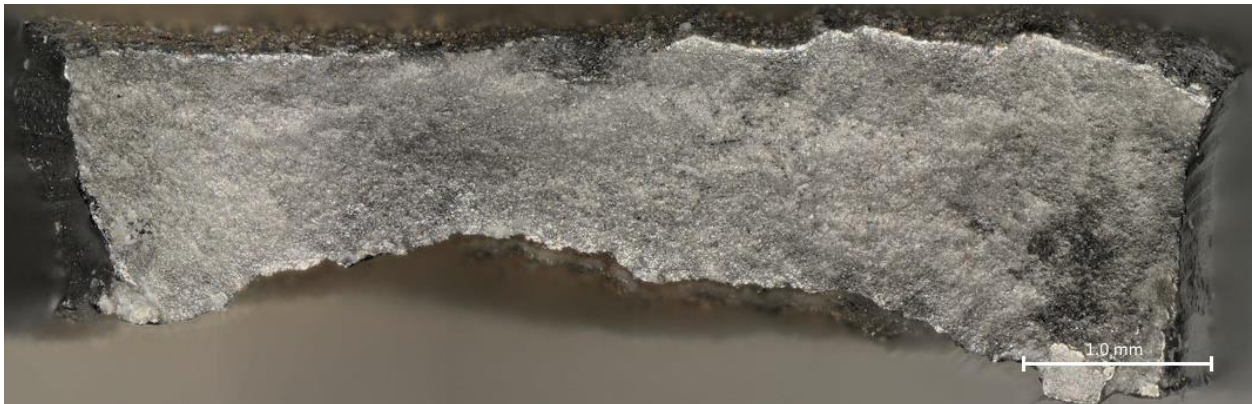
Figure 61: Top-Half Fracture of Control Sample 7A Taken at 100x Magnification
