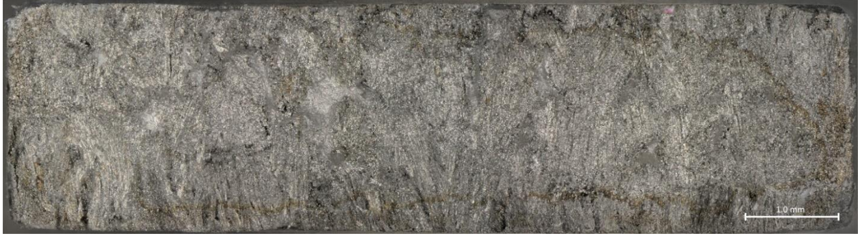
Figure 95: Top-Half Fracture of 43.5-Day Sample 4C Taken at a Magnification of 100x
