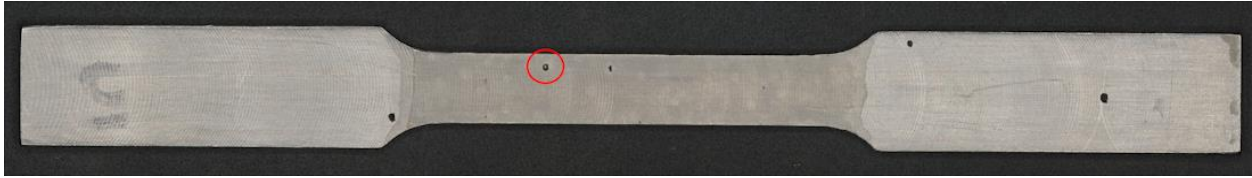
Figure 64: Optical Surface View of 5B's Back Featuring the Tensile Failure Location Circled in Red
