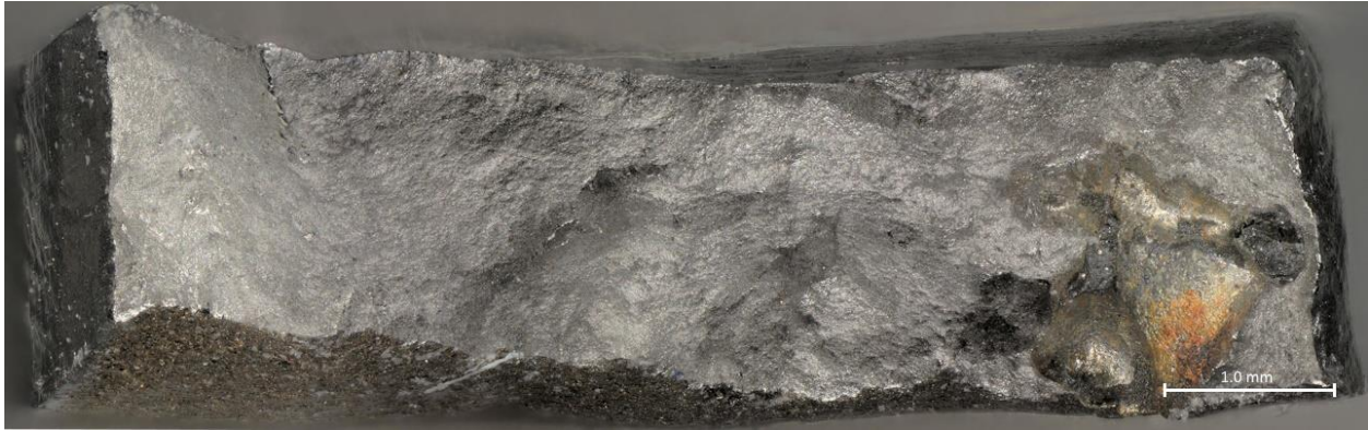
Figure 66: Top-Half Fracture of Control Sample 11C Taken at a Magnification of 100x
