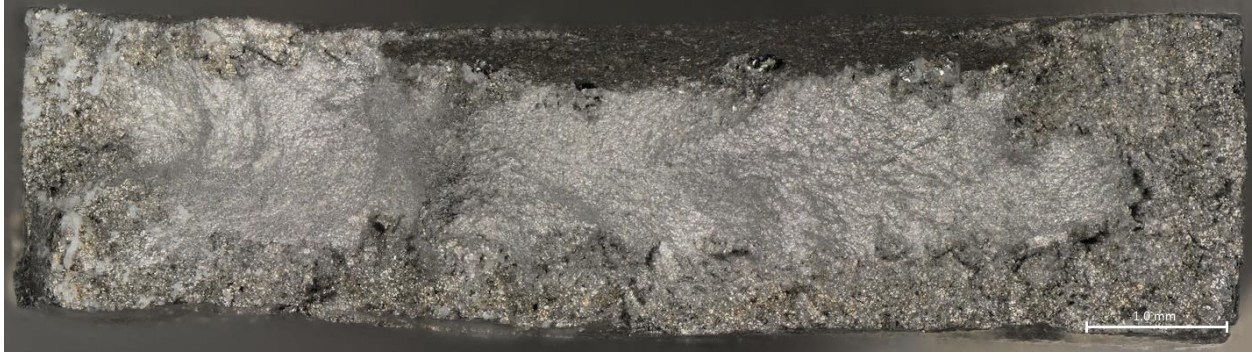
Figure 88: Top-Half Fracture of 43.5-Day Sample 5A Taken at a Magnification of 100x
