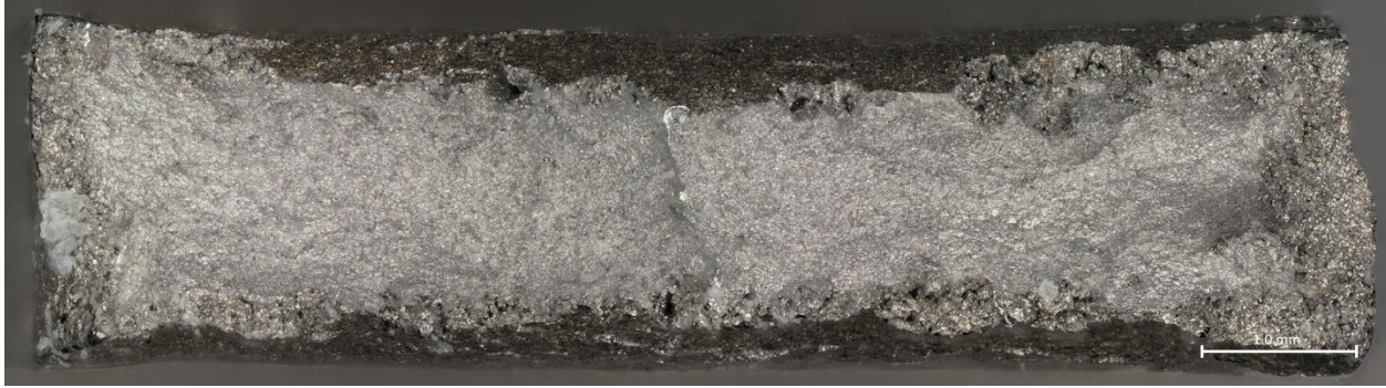
Figure 75: Top-Half Fracture of 21-Day Sample 4A Taken at a Magnification of 100x
