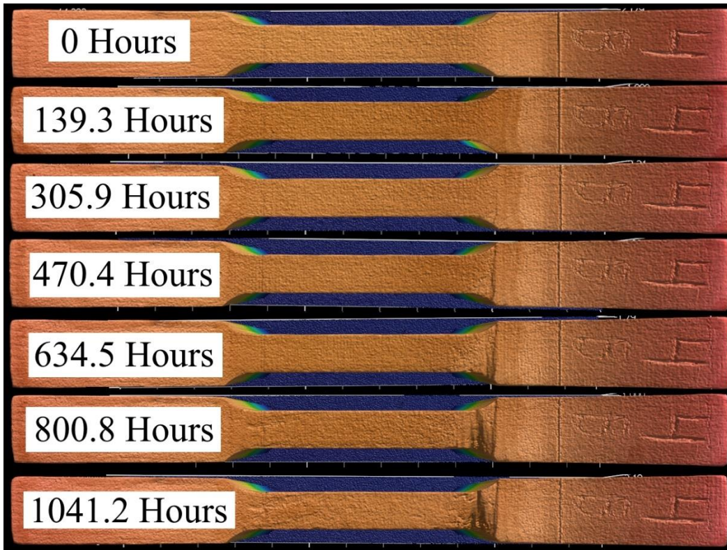
Figure 91: Chronological Progression of 4B's Corrosion Depicted by 3D Topographical Scans
