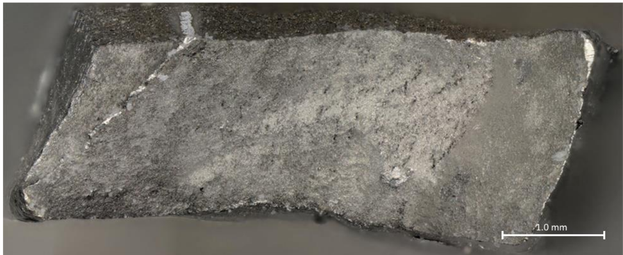
Figure 58: Top-Half Fracture of Control Sample TA Taken at 100x Magnification
