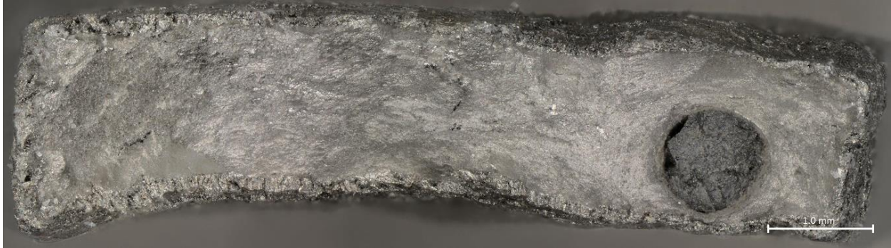
Figure 90: Top-Half Fracture of 43.5-Day Sample 4B Taken at a Magnification of 100x
