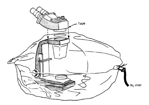
Figure 4.1 Glove bag fitted around a binocular microscope. A hole large enough to fit the eyepiece of the microscope is cut in the top of the glove bag. The glove bag is then fastened to the microscope using electrical tape and purged of atmospheric gases.<sup>20</sup>
