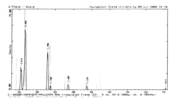
Figure 6.1 Equivalent powder X-ray diffraction pattern for Ca<sub>2</sub>NF obtained after merging 450 frames of single crystal data in GADDS.
