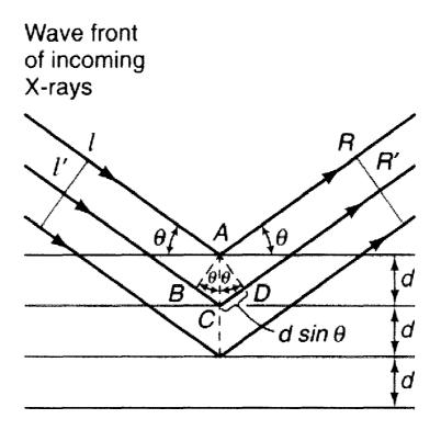
Figure 1.3 Derivation of the Bragg equation,  $2d \sin \theta = n\lambda$ . The diffraction of X-rays may be considered as reflections from different planes.<sup>5</sup>
