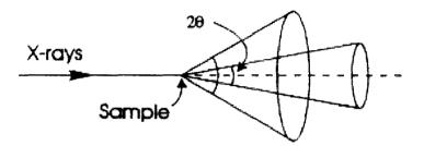
Figure 1.4 Diffraction cones obtained from polycrystalline samples.<sup>1</sup>
