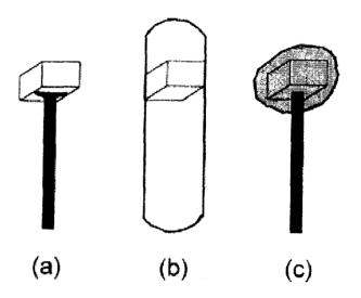
Figure 1.7 Crystal mounting methods: (a) glued to a fine glass fiber; (b) enclosed in a capillary tube; (c) coated with an inert oil.<sup>8</sup>
