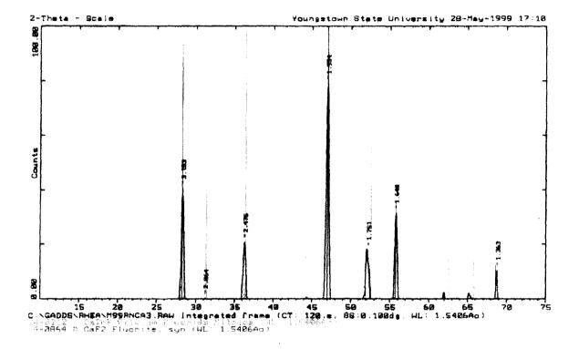
Figure 5.1 X-ray diffraction pattern for Ca<sub>2</sub>NF synthesis product.
