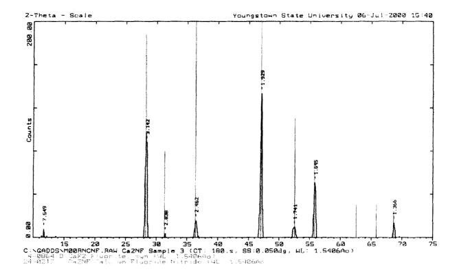
Figure 5.2 X-ray diffraction pattern for Ca<sub>2</sub>NF synthesis product from Trial 8.
