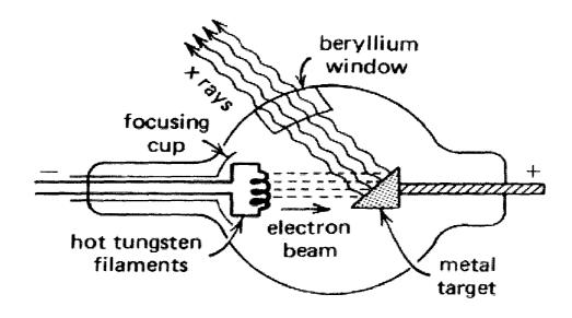
Figure 1.1 Schematic diagram of X-ray tube.<sup>4</sup>
