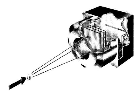
Figure 1.5 Cutaway view of Area Detector. X-rays diffracted from the sample enter the window and ionize the gas mixture. Electronic grids detect the ions and generate electrical impulses which are decoded into position and intensity data.<sup>6</sup>
