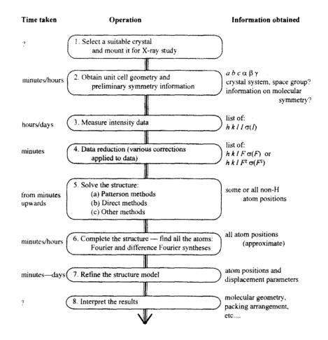
Figure 1.8 A flowchart for the steps involved in a crystal structure determination.<sup>8</sup>
