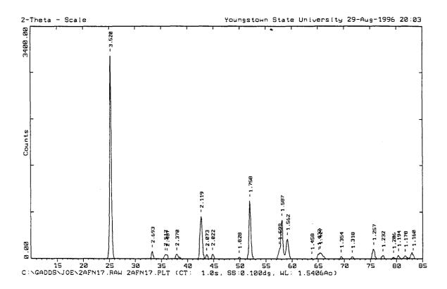
Figure 5.18. X-ray diffraction pattern for  $Al_2(FN)_{1.5}$  synthesis trial 2 product.
