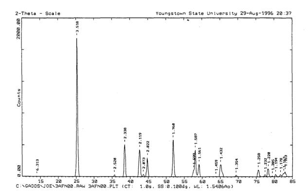
Figure 5.19. X-ray diffraction pattern for  ${\rm Al}_2({\rm FN})_{1.5}$  synthesis trial 3 starting materials.
