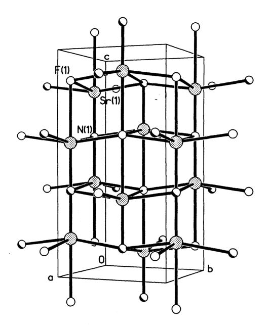
Figure 5.31. Proposed structure plot for  $Sr_2NF$  as calculated by Siemens SHELXTL structure plotting program.
