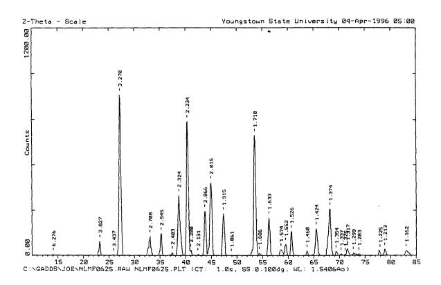
Figure 5.24. X-ray diffraction pattern for  $NaLi_6Mg_6F_{19}$  synthesis trial 1 product.
