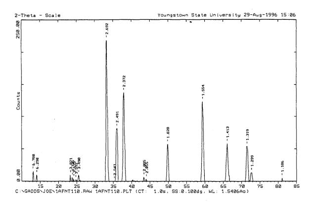
Figure 5.12. X-ray diffraction pattern for  $Al_2(FN)_{1.5}$  synthesis trial 1 product 1.
