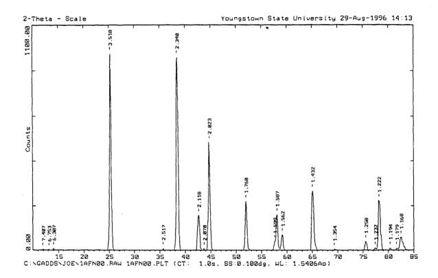
Figure 5.11. X-ray diffraction pattern for  $\mathrm{Al}_2(\mathrm{FN})_{1.5}$  synthesis trial 1 starting materials.
