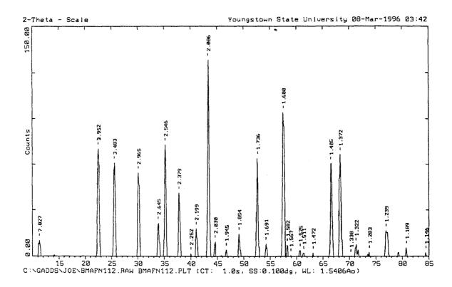
Figure 5.5. X-ray diffraction pattern for  $BaMgAl_{11}F_{10}N_9$  synthesis trial 4 product.
