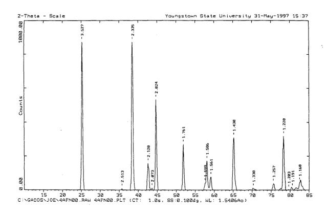
Figure 5.21. X-ray diffraction pattern for  $\mathrm{Al}_2(\mathrm{FN})_{1.5}$  synthesis trial 4 starting materials.
