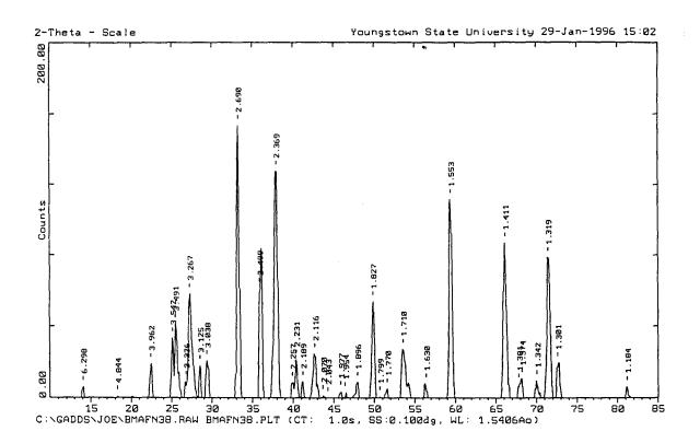
Figure 5.2. X-ray diffraction pattern for  $BaMgAl_{11}F_{10}N_9$  synthesis trial 1 product.
