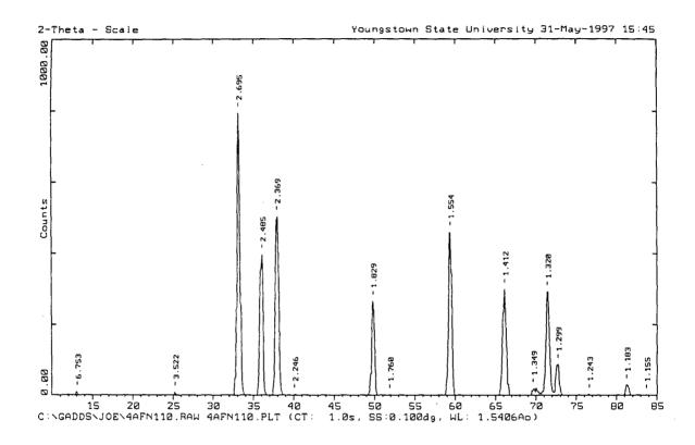
Figure 5.22. X-ray diffraction pattern for  $\mathrm{Al}_2(\mathrm{FN})_{1.5}$  synthesis trial 4 product.
