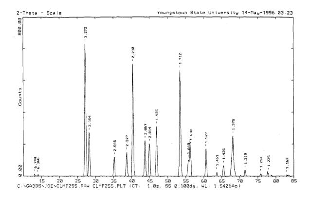
Figure 5.28. X-ray diffraction pattern for CaLi $_5\text{Mg}_6F_{19}$  synthesis trial 2 product.
