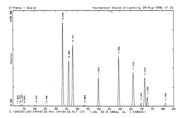
Figure 5.14. X-ray diffraction pattern for  ${\rm Al}_2({\rm FN})_{1.5}$  synthesis trial 1 product 3.
