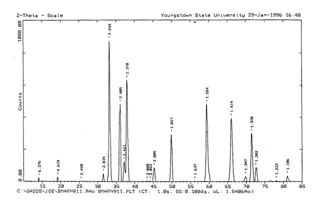
Figure 5.4. X-ray diffraction pattern for  $BaMgAl_{11}F_{10}N_9$  synthesis trial 3 product.
