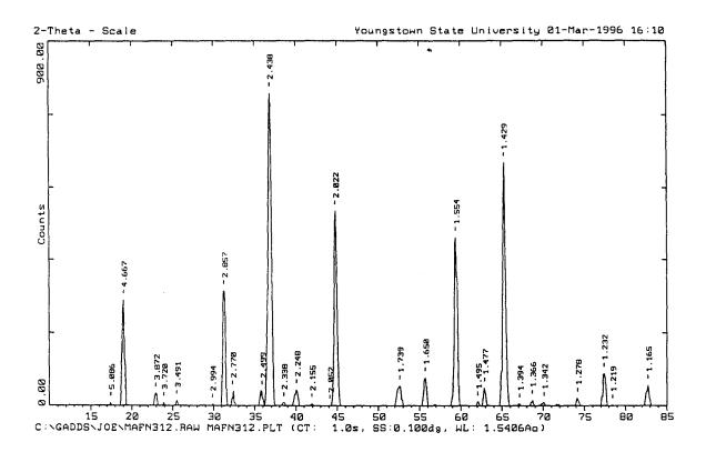
Figure 5.9. X-ray diffraction pattern for  $MgAl_2(FN)_2$  synthesis trial 3 product from nickel boat.
