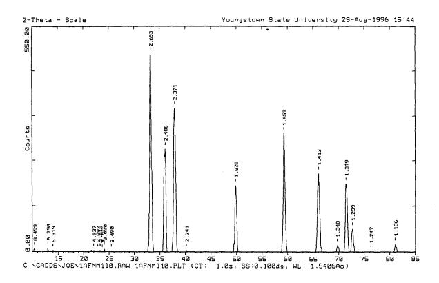
Figure 5.13. X-ray diffraction pattern for  $Al_2(FN)_{1.5}$  synthesis trial 1 product 2.
