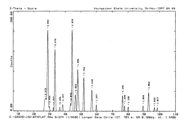
Figure 5.29. X-ray diffraction pattern for  $Sr_2NF$  synthesis product.
