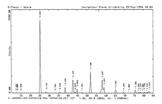
Figure 5.15. X-ray diffraction pattern for  $Al_2(FN)_{1.5}$  synthesis trial 1 product 4.
