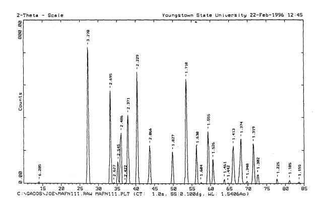
Figure 5.8. X-ray diffraction pattern for  $MgAl_2(FN)_2$  synthesis trial 2 product.
