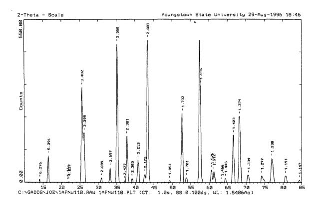
Figure 5.16. X-ray diffraction pattern for  $Al_2(FN)_{1.5}$  synthesis trial 1 product 5.
