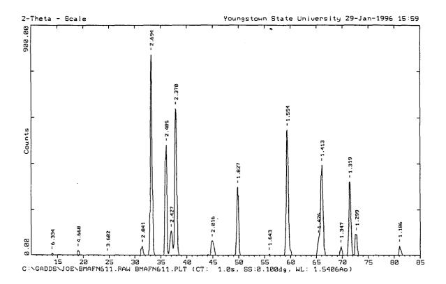
Figure 5.3. X-ray diffraction pattern for  $BaMgAl_{11}F_{10}N_9$  synthesis trial 2 product.
