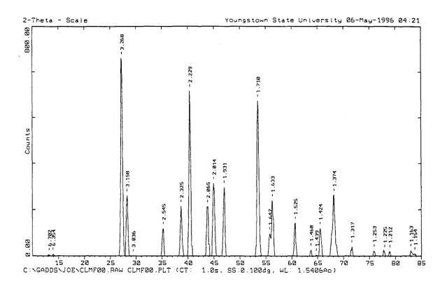
Figure 5.26. X-ray diffraction pattern for CaLi $_5\text{Mg}_6F_{19}$  synthesis trial 1 starting materials.
