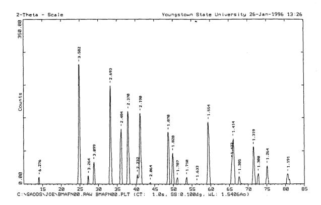
Figure 5.1. X-ray diffraction pattern for  $BaMgAl_{11}F_{10}N_9$  synthesis trial 1 starting materials.
