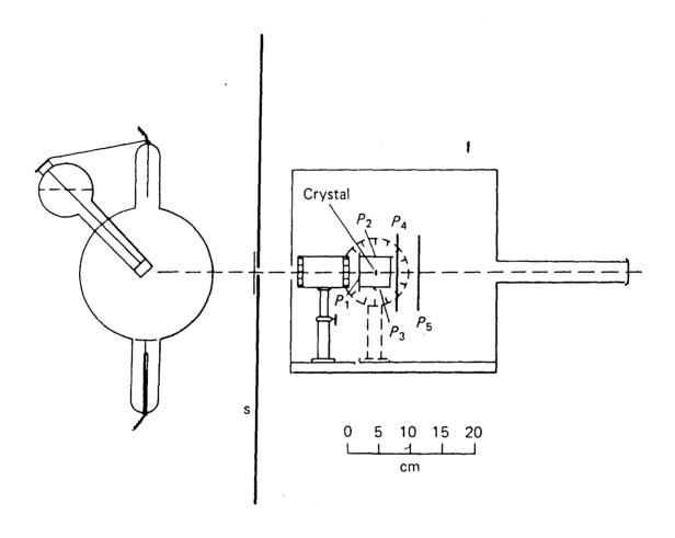
Figure 1.2. Schematic representation of Max von Laue's diffraction experiment, after Bromberg<sup>4</sup>.
