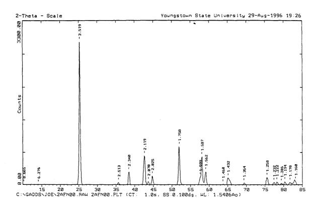
Figure 5.17. X-ray diffraction pattern for  ${\rm Al}_2({\rm FN})_{1.5}$  synthesis trial 2 starting materials.
