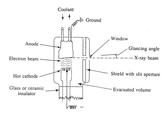
Figure 1.3. Schematic of an X-ray tube, after  $Willard^7$ .
