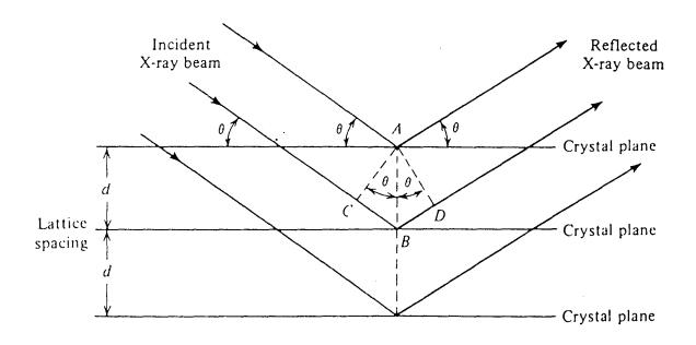
Figure 1.4. Diffraction of X-rays from a set of crystal planes, after Willard 7.
