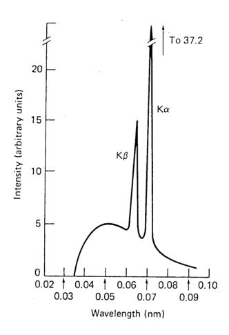
Figure 1.1. Intensity distribution curve of emitted X-rays for a metal, after  $\operatorname{Bromberg}^4$ .
