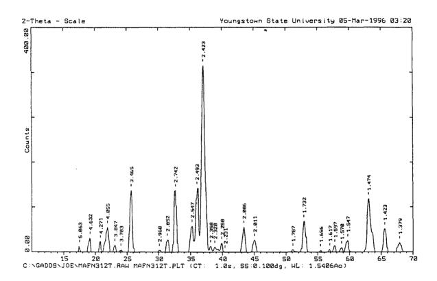
Figure 5.10. X-ray diffraction pattern for  ${\rm MgAl_2\,(FN)_2}$  synthesis trial 3 product from quartz tube.
