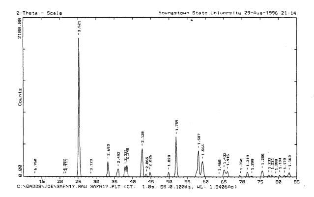
Figure 5.20. X-ray diffraction pattern for  $Al_2(FN)_{1.5}$  synthesis trial 3 product.
