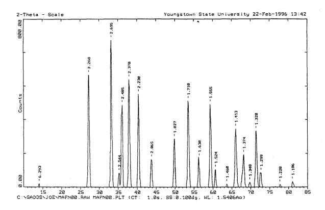
Figure 5.6. X-ray diffraction pattern for  ${\rm MgAl_2\,(FN)_2}$  synthesis trial 1 starting materials.
