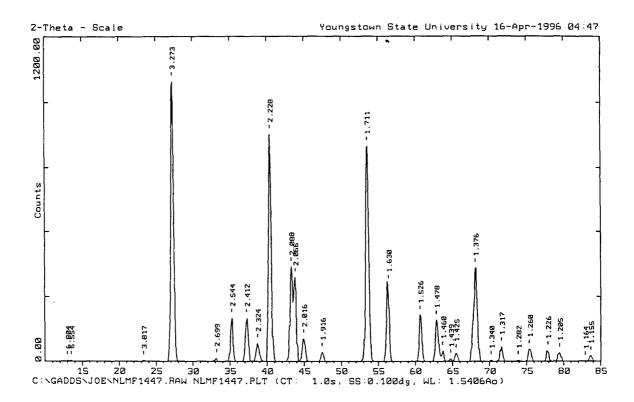
Figure 5.25. X-ray diffraction pattern for  $NaLi_6Mg_6F_{19}$  synthesis trial 2 product.
