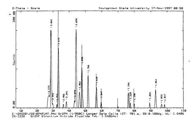
Figure 5.30. X-ray diffraction pattern for  $Sr_2NF$  synthesis product indexed to  $Sr_2NF$  from  $\underline{\textit{JCPDS}}$  database.
