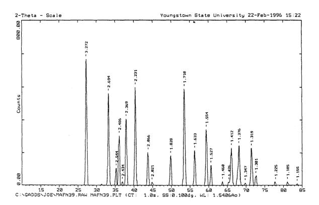
Figure 5.7. X-ray diffraction pattern for  $MgAl_2(FN)_2$  synthesis trial 1 product.
