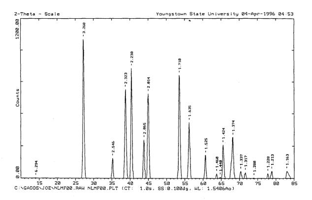
Figure 5.23. X-ray diffraction pattern for  $NaLi_6Mg_6F_{19}$  synthesis trial 1 starting materials.
