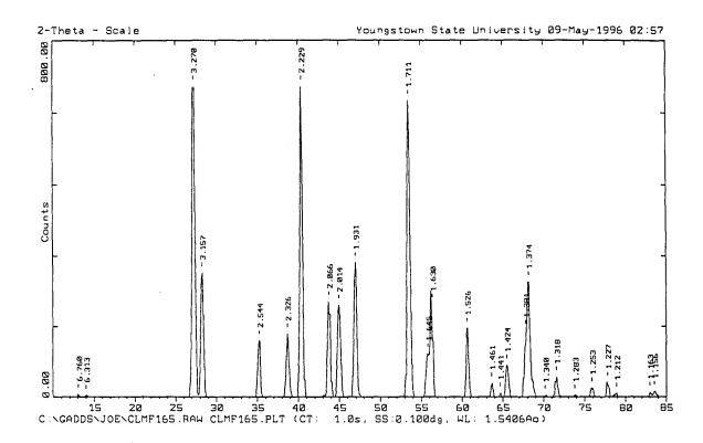
Figure 5.27. X-ray diffraction pattern for  $CaLi_5Mg_6F_{19}$  synthesis trial 1 product.
